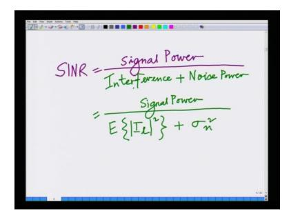
So, now we want to characterize the SINR as SINR equals signal power divided by interference plus noise power equals signal power divided by expected interference power plus the noise signal power divided by interference power is nothing but expected I l square plus sigma N squared which is the noise power. Now, let us start characterizing each term that is first I want to characterize signal power then the interference power then the noise power.
