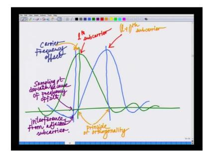
And then with that, we had moved on the effect of frequency offset, what is the distorting effect of frequency offset in OFDM system? We said OFDM divides the frequency band into a set of orthogonal overlapping yet orthogonal frequency get us. The orthogonality is a very critical aspect actually of any OFDM system which means once you have an OFDM system as we had depicted in this figure last time. The orthogonality is lost which means now there will be ICI or inter carrier interface.
