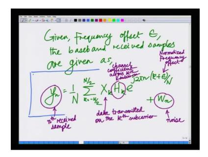
We had set for a frequency offset of epsilon, normalized with respect to sub carrier bandwidth. The received signal sample y n is given as summation X k H k e power j 2 pi N k plus epsilon over capital N number of sub carriers plus noise that is we said the system model for this.
