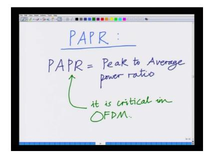
So, I want next issue I want to address in this context is the PAPR issue in OFDM. This is the PAPR issue in an OFDM system. What does PAPR stand for? PAPR stands for PAPR equals peak; it requires peak to average. PAPR stands for simply stands for peak to average power ratio and simply put this is a critical this is a critical factor in OFDM. This is critical, this is critical in an OFDM system. What does this PAPR issue for instance? Consider a typical non
