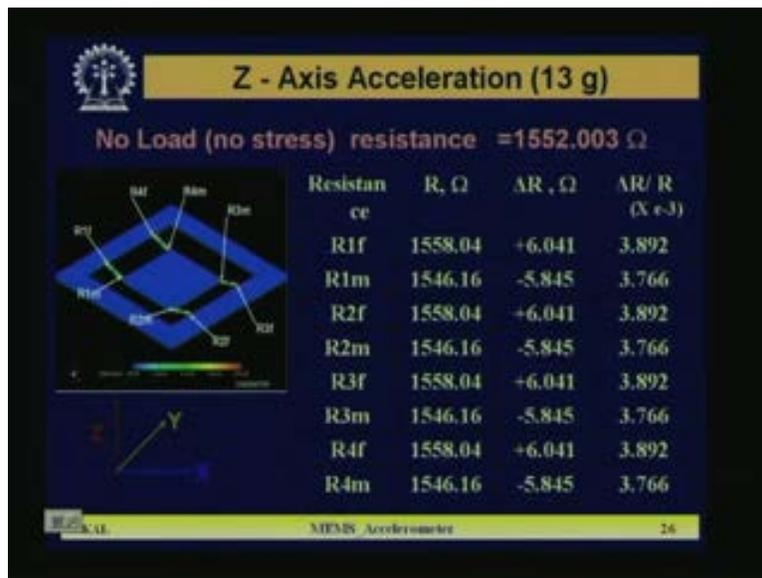
But here the change of resistance valued values for Z acceleration, no load stress. Here is a 51.5 kilo ohm and here the resistances are R1f 1m all the same kind of location we have used and there you can see the values delta R by R you can see 3.892. Here in 3.892,
