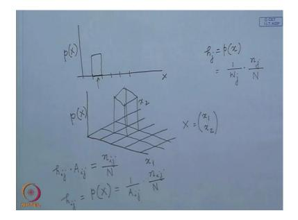
So, if I have variable X, and on this axis I plot the probability density function p X, then what we have done is the X axis is divided into number of beams and number of cells. And within a cell we have assumed that the probability function is constant, so it is
