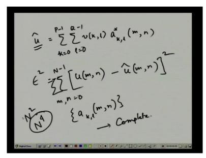
And it can be shown that this approximate reconstructed image will enca will have an error a limited error if the basis matrices that we are considering the set of basis matrices or set of basis images that is complete. So this error will be minimized if the basis images that we consider is complete basis images. So in that case what we will have is the reconstructed image that u hat will be given by double summation say v(k,l) into a\*k,l(m,n).
