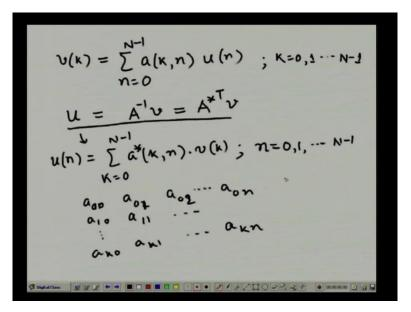
If I expand this, so now what I do is, I expand this matrix equation. So if I expand this matrix equation this can be represented as a series summation which will be given by v(k) is equal to a(k,n) into u(n), where n varies from 0 to capital N-1.
