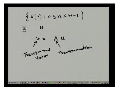
So the series of samples can be represented by say u(n) where 0 less than or equal to n less than or equal to capital N-1. So we have a series of discrete samples u(n), so in this case we have capital N number of samples.
