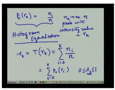
So here, in case of histogram equalization, if I consider a discrete case, in a discrete case we have seen that the histogram of an image is given in the form like this, that is Pr(rk) where rk is an intensity level present in the image, and which is given by summation of ni by n, i varying from zero to k where n k, is the number of pixels with intensity value is equal to rk, sorry this is not summation Prk is given by ni by n.
