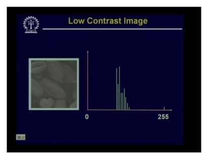
Then the next image shows, that here the image has got in pixels having intensity value in the middle range, but the range of intensity values is very narrow. So as a result, the image is neither very bright nor very dark, but at the same time because the dynamic range of the intensity values is very low, the image contrast is very poor.
