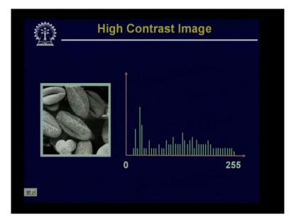
So as the next slide shows, which we call a high contrast image, where you find that most of the details of the objects present in the image are visible, and by looking at the corresponding histogram, we find that the pixels in this particular image have wide range of intensity values starting from very low value which is near about 0 to the maximum value which is near about
