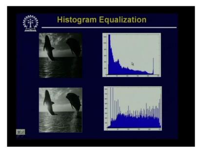
So here we have shown on image which is a very very dark image, and on the right hand side we have the corresponding histogram, and once we do histogram equalization, then what we get is an equalized image or the processed image, and on the bottom row you find that we have a brighter image which is the histogram equalized image, and on the right hand side, we have the corresponding histogram.
