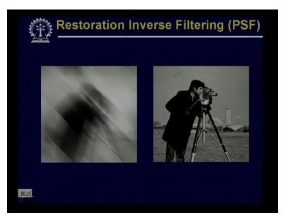
Now if I perform the inverse filtering using this recomputed degradation function then we find that the reconstruction result is very very good. So this was the blurred image. This is the reconstructed image during by using the inverse filtering direct inverse filtering, but here the degradation model was recomputed from the point, from the Fourier transformation of the point spread function.
