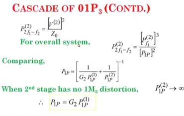
This relation transfers P1P between input and output of a RF block
