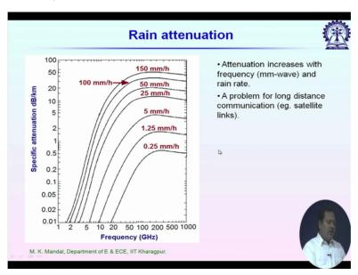
So not only that fog, rain and sand storm, dust storm so all of these weather condition also affect millimeter wave propagation. So this is a typical attenuation plot umm with rain rate with difference frequency range so if you follow any one curve so lower rain rate for example .25 millimeter per hour to 1.25 millimeter per hour.
