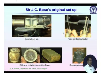
So in this slide you can see the different component used by Professor JC Bose this bottom right corner it shows this spark gap so we have two gaps between this two pin. High voltage is applied between these two pins which generate sparks so sparks it content a white electromagnetic spectrum starting from optical wave to RF.
