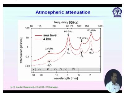
So but millimeter wave communication it has to face many challenges so one of them is atmospheric attenuation. So this figure typically it shows the attenuation in db per kilometer versus the wavelength. So if you look at the diagram we have a solid line and one dotted line so this dotted line it corresponds to the measured attenuation in db per kilometer at a 4 kilometer height from the sea surface sea level.
