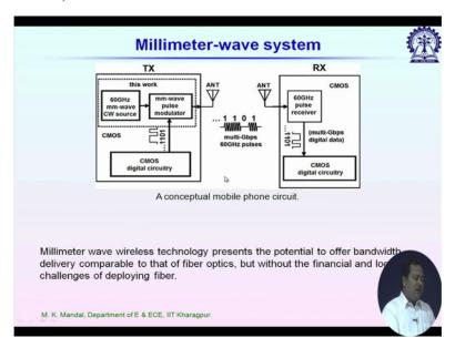
So this is a typical RF umm millimeter wave transmitter and receiver circuit there is conceptual diagram. So in the transmitter circuit you can see that we have a 60 gigahertz millimeter wave continuous source. So which is being modulated by the base band its coming from CMOS digital circuitry. So the cost of any millimeter wave system it depends on fabrication procedure.
