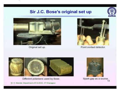
And then you can see the transmitting part here so inside we have the spark gap so from which electromagnetic wave is being transmitted by this pipe now we call it horn antenna. So this is a prism made of dielectric material so to show the refraction property of electromagnetic signal and this is the reviver side. So at the receiver you can see top right figure so we have a point contact detector so this is it.
