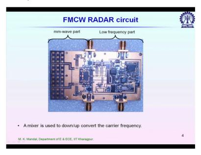
So if I, Let us just look at a circuit millimeter wave circuit. So this is a millimeter wave circuit which is fabricated on a printed circuit board. You can see the black color dielectric material and the shiny is the copper. So if I look at the left hand side it has actually two parts. One high frequency component parts which is millimeter wave frequency component parts and in the right hand side this is the low frequency component parts.
