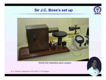
So this an replica of the original system design by Professor JC Bose in Kolkata. So you can see this a box so inside this box we have millimeter source which is nothing but a spark gap and then he used a tube metallic hollow tube as the transmitter now we know that it behaves as an antenna and we have a (())(25:33) table here.
