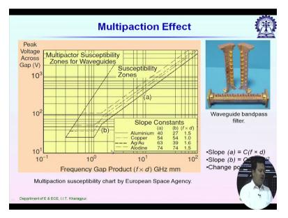
Now how to predict multipaction or what is the threshold voltage needed for multipaction? Its really difficult to calculate the multipaction threshold voltage because it depends on many factors. It depends on type of metal because the secondary emission threshold energy needed for secondary emission it depends on type of metal, surface of metal and presence of any other molecule inside the rectangular waveguide structure.
