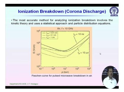
Now lets consider one interesting thing.Lets say we are testing a waveguide bandpass filter and its design in rectangular waveguide technology now ionization breakdown may happen or multipaction breakdown may happen so from this structure under test how do we understand which breakdown occurs fast so once a breakdown happen after that we open the structure.
