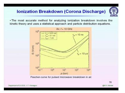
So we have a curve here for umm the threshold electric field value versus pressure plot this is called paschen curve for pulse microwave breakdown in air for different L effective values. L effective will changes with of course pressure so L effective this is sorry L effective it depends on the type of molecules or the type of gas inside.
