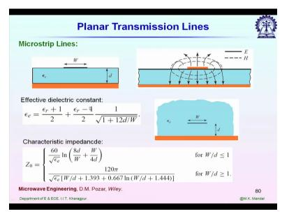
So if I go back this first figure it shows a cross section of a microstrip line. So we we have a top strip metallic strip. It sits on a dielectric layer and below we have a ground plane. This is the plot of electric field and magnetic field. Most of the electromagnetic energy it lies its confined inside the dielectric and below this strip we have some flanging field in air so these are semi opened structure.
