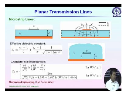
So after this rectangular waveguide next will start the printed lines. So among the printed lines most popular even at millimetre wave frequencies are microstrip line and CPW line. For microstrip line and CPW line what we expect that loss alpha value will be much more compare to rectangular waveguide and then what is the use of microstrip and CPW line?
