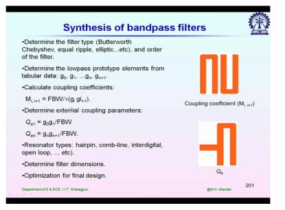
And for this left-hand side figure, it is always mixed coupling and the coupling coefficient you see it decreases with increase in separation. Now, once you have this plot so in the synthesis state if we go back you see, we will be having different M ij values that nothing but coupling coefficient with different resonators, so you can then calculate what is the gap required between 2 resonators for the required coupling coefficient from this matrix.
