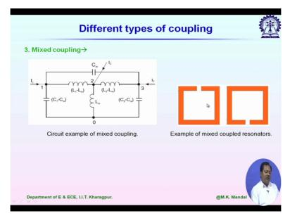
Sometimes we may face mixed coupling, so coupling is let us say for this example, it is due to both electric field and magnetic field and sometimes what happens for some given gap let us say not for this example, I have some other example, yes this one.
