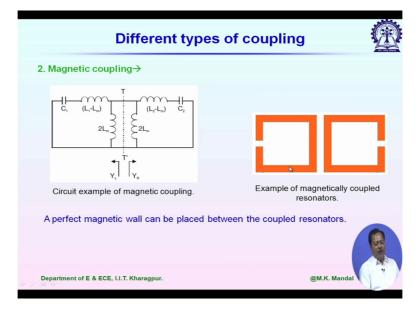
So the orientation of electric field is different and if I consider a symmetrical plane in between, it can be shown that electric field direction is perpendicular on that and it behaves like PEC and it is electric coupling. So, for a coupled resonators system so we have 2 frequencies, if at lower frequency it is electric coupling this coupling is due to electric field, we call it electric coupling and the lower frequency, it is due to magnetic field then we call it simply magnetic coupling.
