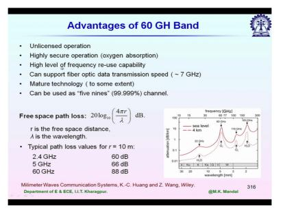
So what are the advantages of 60 gigahertz band, first of all throughout work it is unlicensed band 57 to 63-64 almost 7 gigahertz this is unlicensed band and highly secure operation is
