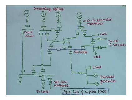
So, if you take like these are all small rectangular boxes are. So, on this are basically circuit breakers, right. And suppose you have a generating stations this is generating stations.
