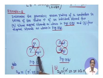
But look at this example figure, I will show you determine the geometric mean radius of a conductor in terms of the radius r of an individual strand for a these 3 equal strands as shown in figure 19 a and b 4 equal strands as shown in figure 19 b right. So, this is your figure 19 b right.
