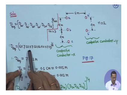
So, it is 6 into 7.11 into 7.11 into 6 into 10 into 7.11 to the power 1 upon 6. It will come 7.162 meter right. Similarly r x the group x right. All the radius your diameter same 0.2, for this one, this one, this one. So, radius will be 0.2 by 2 that is 0.001 meter. Similarly here also this group radius is diameter is 0.4 centimeter. So, r y is equal to 0.4 by 2 is equal to 0.2 centimeter is equal to 0.002 meter right.
