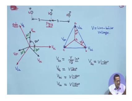
This angle will be 30 degree just now I showed this angle will be 30 degree. And is line to line voltage So, this line will be V ac line to line voltage lagging from V an by minus 30 degree all these things are known and line is untransposed right; that means, that is charged expression of charge will become complex right. So, now, apply equation 5 again you have to go back to equation 5.
