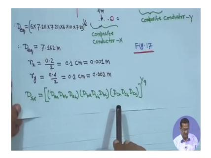
Therefore find out yourself one with the self G md 1 for this group for this group right. Therefore, D sx, D aa, D ab, D ac, D ba, D bb, D bc, D ca, D cb, D cc. D aa, D bb and D cc actually is equal to r x. And all the 9 possibilities 3 into 3. So, to the power 1 upon 9 right. (Refer Slide Time: 08:25)
