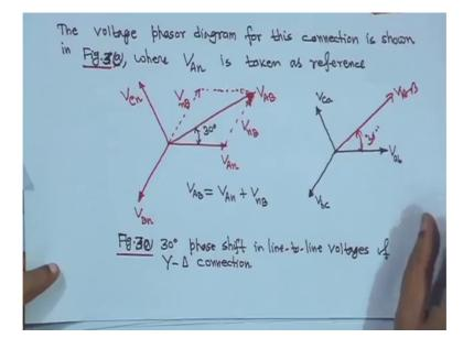
So, so we have seen that line to line voltage right, on the star side leading the line to line voltage delta side by angle 30 degree right. We will come to the per unit slowly and slowly.
