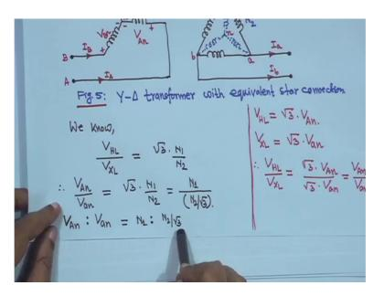
This much you have understood? Therefore, this V HL upon V XL V HL upon V XL is equal to V AN upon V AN; that means, this V AN V capital A N upon V AN is equal to root 3 into N 1 upon N two; that means, it is N 1 divided by again we are writing N 2 upon root 3 that is V AN is to V AN is equal to N 1 is to N 2 upon root 3. As if this turn was N 2 I mean meaning is something like this.
