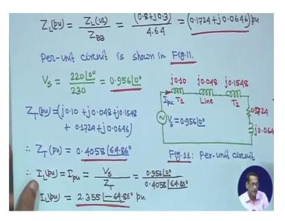
That means section 3 base impedance you have obtain Z B 3 is equal to 4.64 ohm this one, this one right; that means, your per units your Z l is equal to your Z l ohm upon Z B 3.8 plus j 0.3 upon this is 4.64 that is 0.1724 plus j 0 0.0646 per unit right.
