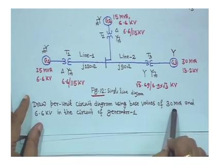
So, this is actually your before giving the data this is actually your figure 12, figure 12 there are 3 generators - generator 1, generator 2 and generator 3 right. Now this generator 1 this stars are connected it is grounded, generator 3 is not grounded, generator 2 is grounded.
