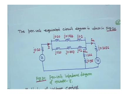
Therefore per unit equivalent circuit diagram is shown in figure 20 that mean these diagram right, this is generator then you have 2 parallel lines transformer then line then again transformer 0.2, 0.1033, 0.22, again this and for other line this is j 0.2 because all transformer per unit was same.
