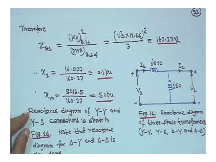
Therefore, Z B 1 is KV square base line to line by MVA base 3 phase that is root 3 into 12.66 square upon 3 that is 160.27 ohm therefore, x 1 will be original earlier we got x 1 is 16.027 ohm and x m is 8013.5 ohm therefore, x 1 will be your 16.07 upon 1027 upon 160.27 is equal to 0.1 per unit.
