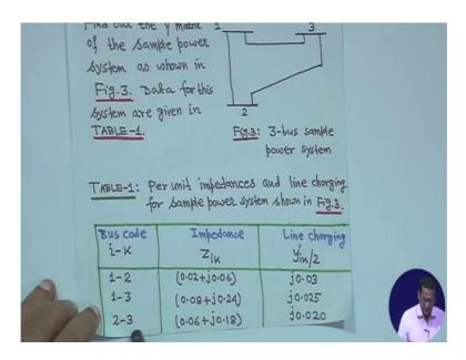
So, this is 1 2 3, the 3 bus problem and generator are thing nothing shown only 1 2 to 3 all this things are given right. So now, the charging admittance we have taken an how charging admittance will included I will tell you right. So, this is the bus code they write bus code that is I mean current sending and receiving and bus i to bus k right. So is so, it is just one end to another end one bus to another bus.
