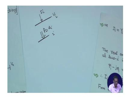
Suppose this is my, this is my bus bar this is my bus bar, this is the voltage V i right. We are taking this is the current injection actually I i right. So, this way you are taking basically any bus bar if you take any bus bar if you take i th bus bar right. So, I am putting like this that power injection is I put like this real power is P i and k power injection is Q i in this bus right.
