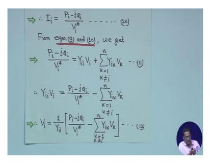
That means, we can write Y I i V i is equal to i means this term is equal to this term first minus this term. So, P i minus jQ i upon V i conjugate minus k is equal to 1 2 n capital Y ik V k, k not is equal to i right. So that means, V i is equal to V i is equal to 1 up on capital Y I i in bracket, P i minus jQ i divided by V i conjugate right. Minus k is equal to 1 2 n capital Y ik V k, k not is equal to i, this is equation 12 right.
