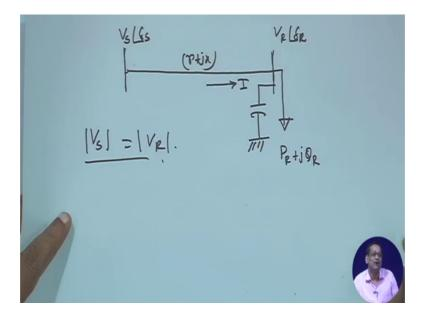
This one you will do of your own for example, this is sending and voltage and this is your receiving end this is sending end this side voltage you say V S and its angle is delta s right this your this thing and this side is V R and angle is delta R right and this line impedance say I am putting this small R j exist or total impedance of the line the resistance the reactor right and this side load is there load is there at the receiving end this is P R plus j QR right.
