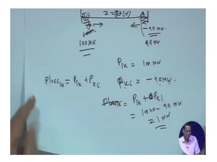
Suppose you have a bus bar suppose you have a bus bar this is have a i-th bus and this is k-th bus right suppose at this point suppose the line has the impedance z is equal to your R plus jx line has the impedance right. So, at this point if you suppose power flowing is these direction right. So, and this side you take this direction. So, at this point you measure the power right.
