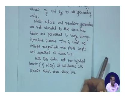
And this is must as voltage magnitude and phase angle are specified at slack bus this is known with this data net bus injected power Pi plus J qi at all buses are known after the other than the slack bus if it is I mean if all buses are P Q buses right. So, this is the first step that all the data you have to prepare.
