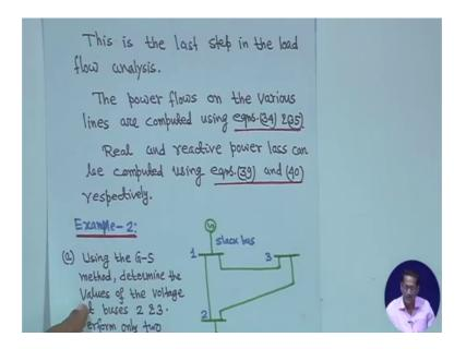
So, this is equation 34 and 35 and real and reactive power loss for the line can be computed using equation 39 and 40 that also we have shown know P loss ik and Q loss ik equation 39 and 40. So, that way also you can you can solve it right.
