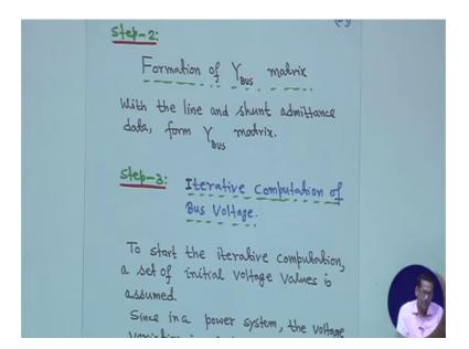
Second step is form the Y bus matrix that is line parameters are given. So, second step is that you have to form the Y bus matrix right then third step is the iterative computation
