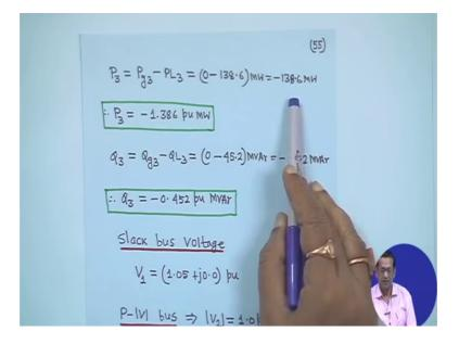
So, similarly P 3 is equal to Pg 3 minus PL 3. So, that is no generi that is no generator at bus 3 sothis 0 minus 138.6 megawatt that minus 138.6 megawatt. So, it is divided by 100, I am not dividing it 100, but if you divided by 100, it is h100 mb is the base so minus 1.386 power unit megawatt right. Similarly per Q 3 is also Qg 3 minus QL 3 is minus 45.2 megawatt so divided by hundred it will be minus 0.452 power unit megawatt. A slack bus voltage is same 1.05 plus j 05 and 0 right.
