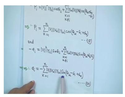
So, this one your equation 16 and n is equal to 3, this is equation 16 then n is equal to 3 because at bus 2 it is your Pv bus. So, in that bus your what you call Q 2 is not known right. So, we have to see that how iteratively you can made it right. So, what you will do
