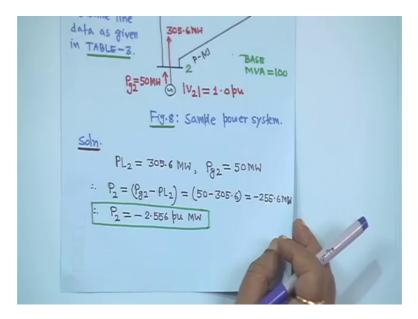
And reactive load is 45.2 megawatt right and this bus is a Pv bus, this bus is a Pv bus. So, here for bus 2 voltage magnitude is specified a Pv bus P has to be specified and voltage magnitude has to be specified. So, voltage magnitude V 2 is equal to 1.0 per unit it is specified. And they load that is 305.6 x megawatt Pg 2 is also 50 megawatt, but you
