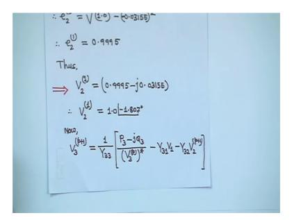
So; that means, it will become e 2 1 that is 0.9995, then you will take V 2 1 actually 0.9 triple 95 minus j this 1, this will give you magnitude one because based on that only got this e right and it a angle is be minus 1.807 degree that mean this one this one using Q 2 injection that is we got 0.98396 and minus j 0 0.0315, but corrected value we corrected right.
