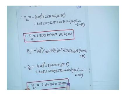
It is positive means power is flowing 1 to2 right and here at the P 21 it is minus 174.4 megawatt, then the power actually flowing from why your what to you call one to two, but is P 21 is showing minus right that mean P 2 in one this one, this one is your P 1 to this one is 1 8, this is one is 181.89, it indicate difference indicate that resistive lose in the in the line right that we will see after this.
