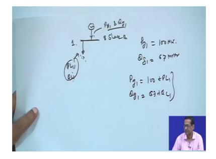
So, I told you once that if slack bus is there the slack bus is there suppose this is your slack bus this is your slack bus right. So, generator is here right suppose bus one is a slack bus. So, just hold one. So, bus one is a slack bus right and in that case your this P g 1 and Q g 1 are computed actually when solution has converge.
