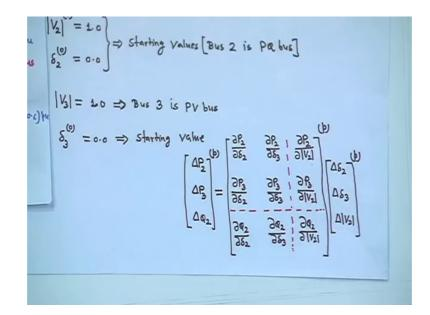
So, this is delta P 2 upon delta delta 2 delta P 2 upon delta delta 3 delta P 3 upon delta delta 2 delta P 3 upon delta delta 3 this is delta delta 2 delta delta 3 and this P actually for iteration count right. So, as bus voltage magnitude is fixed that is V 2 is your magnitude 1.0. So, there is no question of delta V 2 iterative process delta V 2 will never come because this voltage magnitude here is fixed at one per unit at one per sorry at bus 3 that voltage magnitude is fixed.
