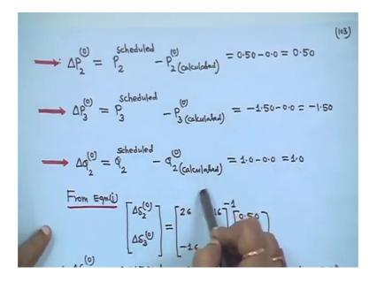
Therefore, delta P 2 0 is equal to P 2 schedule minus P 2 calculated. So, that is 0.5 minus this one this is 0.5 is step I am showing you such that you can understand actually the flow of your algorithm right and delta P 3 0 will be P 3 schedule minus P 3 0 calculated.
