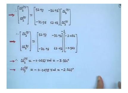
And this is delta delta 2 0, delta delta 3 0, for the pi 0 3 I mean P is equal to 0 that is initially that is your in that way you can say this is the first iteration actually right then the delta delta 0 delta is a 0 is equal to this matrix inverse. So, 52.97 minus 31.98, this 1 minus 31.98 63 point be inverse then minus 2.056 and minus 0.946.
