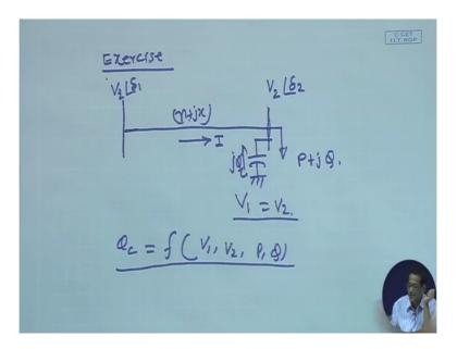
For example: this is an exercise for you. Suppose you have all these things will study, but in advance I am giving. Suppose you have a transmission line this side is sending end, this voltage is say V 1 angle delta 1, this side is receiving end is sending end voltage V 2 delta 2, this impedance of the line is r plus j x, current flowing through this line is I and here you have load P plus j Q; this is the load.
