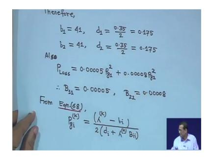
when you take the derivative this one actually it is b 1 plus 2 d 1 which is b 1 plus your B 2 plus 2 d 2. So, 2 d 1 is equal to 0.35 here also 2 d 2 is equal to 0.35 that is why d 1 is equal to 0.35 by 2 right.
