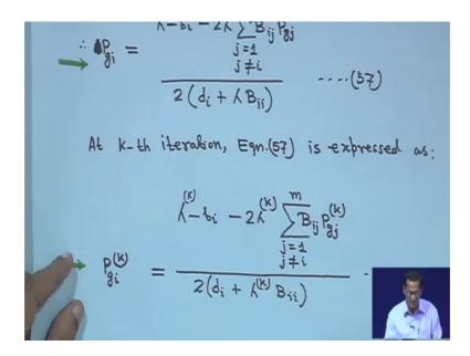
Then from this equation you can write lambda; from this equation you can write Pgi is equal to lambda minus B i minus 2 lambda this whole term divided by 2 into di plus lambda Bii. This is equation 57 right. now your k th iteration this equation 57 is expressed, as just put Pgik just put Pgik here this bd all are constant right that is equation 58 this is Pgik if you take the summation of this Pgik that will be your total load.
