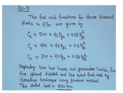
500 plus 41 Pg 1 plus 0.15 Pg 1 square C 2 is given 400 plus 44 Pg 2 plus 0.1 Pg 2 square. C 3 is equal to 300 plus 40 Pg 3 plus 0.18 Pg 3 square right. You neglect the line losses first you will neglect the loss right and generator limits, generator limit is also not there we will consider in the next problem right you have to find out the optimal dispatch and the total fuel cost by iterative technique using gradient method, total load is 850 megawatt right that is the thing.
