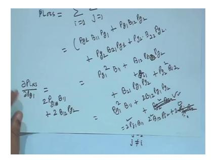
So, it will be 2 Pg 1 B 11 I am just writing, say it in this case a del P loss by del Pg 1 is equal to 2 Pg 1 B 11 plus 2 B 1 2 Pg 2 right.
