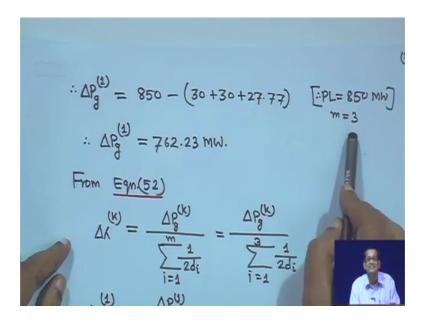
Now you have to mismatch you have to make it delta Pgk is total load minus total generation this is the formula. So, at first iteration you find out what is the. So, in the first iteration when k is equal to 1 delta Pg 1 is equal to 850 minus 30 plus 30 plus 27.77 right total load is 850 megawatt written here right and m is equal to 3 generators are there; that means, delta Pg 1 is equal to 762.23 large difference. So, you have to go for the next iteration.
