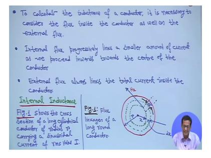
Next is to calculate the inductance of a conductor it is a necessary to consider the flux inside the conductor as well as the external flux both internal as well as external both the flux linkages we have to considered to determine the inductance of a single conductor right current carrying conductor.
