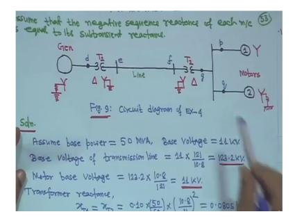
Now this one for this transformer positive sequence only this impedance for transformer. So, j 0.0805 remain same for negative also in this see that, then this j 0.33 that your this that one is coming for your transmission line, this is for transmission line; that means, this is the line next line will come transmission line.
