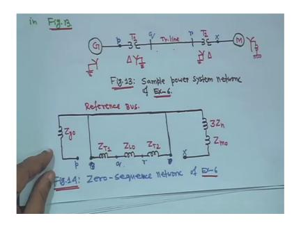
So, connect it and here star is grounded connected, but this is delta this is star isolation is there. So, it cannot be connected. So, this is the 0 sequence network for this kind of for this network. Next one is that figure 15 actually this is a double circuit line look it.
