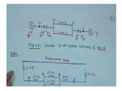
So, this is all parameters are given you have to draw the 0 sequence diagram. In this case in this case same thing, but no delta or star delta transformer. So, it is star grounded star grounded star grounded all star grounded, but this is ungrounded that motor. So, reference bus you will take.
