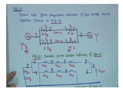
So, you have a generator star grounded you have a point mark here p l m n e q g a f u all I have marked you mark of your own. This is delta star transformer star is grounded. This is star delta it is ungrounded delta star transformer star is grounded, but this here star is grounded delta transformer, but here star is not grounded and here it is star.
