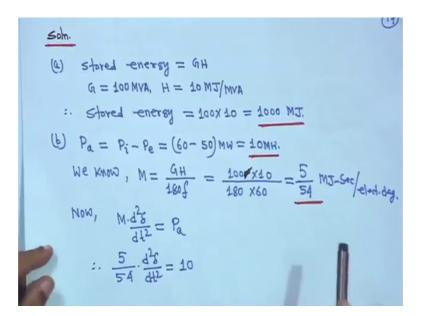
So, accelerating power actually 10 megawatt; now we know M is equal to G H up on 100 80 f that is we are putting mega joule second per electrical degree. So, G H is equal to 1000 into your 10; your one it is actually 100 here, it is 1 here, H G is actually 100; I have made a mistake it is 100 into 10, but this answer is correct 100 into 10 divided by 180 into 60 that is 5 by 54 that is mega joule second per electrical degree.
