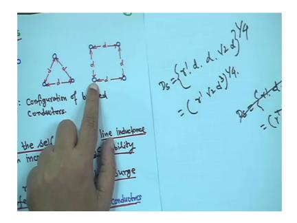
Say D s this is for 4 conductor case and this diagram D s is equal to first you will take the self one r dash then you take the distance from this conductor to here it will be d then this conductor 2 to here it will be d and then this conductor to that this is d, this is d. So, this distance diagonal distance will be root 2 D to the power 1 by 4.
