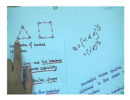
So, suppose this D s is take any conductor D s is first you will take its r dash right then from here from this conductor take the distance of it that is in d and this conductor again you take the d right assuming all the conductors have the same radius r
