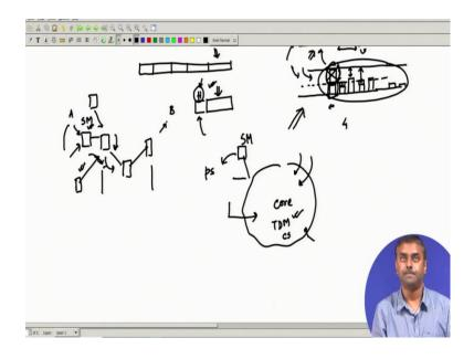
So, I have a network, let us say I have some node A that wishes to connect to B ok? So, it is geographically separated and A wants to communicate to B, A generates this kind of data traffic which is bursty in nature and it is targeting B. Now of course, in networking, we know that directly I do not give a copper wire or something fiber wire or wireless link from A to B, we go through networking we put switches and all those things.
