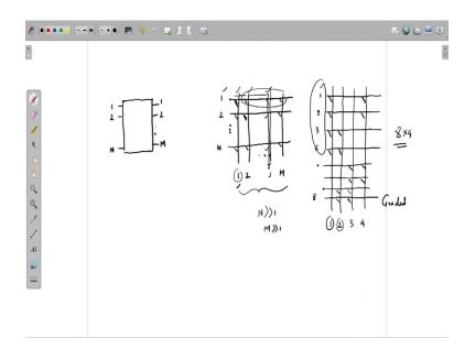
Now, M trunks are there, ok. What is the connectivity? Again, I can construct a crossbar switch. At the output, I will be taking because M number of outputs are required. If I provide these connectivities, it is good enough.
