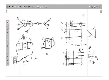
So, first, what they do is they try to connect to the local subscriber loop. And from there, we have already shown this diagram that it goes to some trunk where multiple such local subscriber loops connect to, ok. And then it goes via multiple trunks in between, and then finally, it gets connected to again some subscriber over here, ok.
