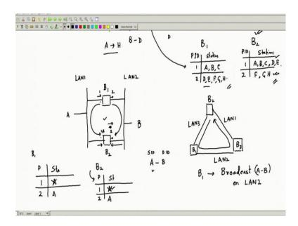
So, let us try to see suppose we have 2 bridges, bridge 1 and bridge 2 connected to the same LAN. So, this is LAN 1, this is LAN 2 ok.
