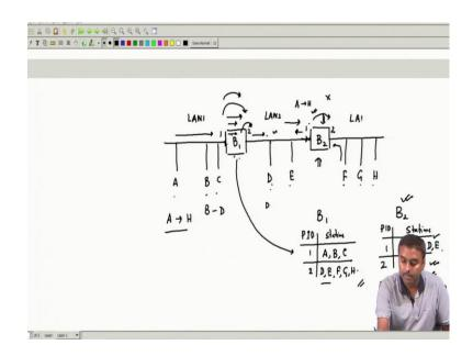
So, let us say instead of this 2, I connect multiple LANs with 2 bridges, bridge 1 and bridge 2. Station A and B, let us say C is connected over here, D and E are connected over here, and F G, and H are connected over here. Now, what will happen to the learning bridges? Let us try to understand that.
