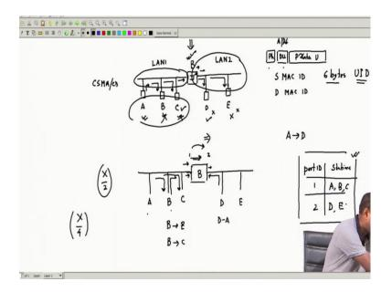
So, let us say the same LAN scenario A B, and C are connected, over here D and E are connected. So, let us say the first packet A to D is coming to the bridge after broadcasting.
