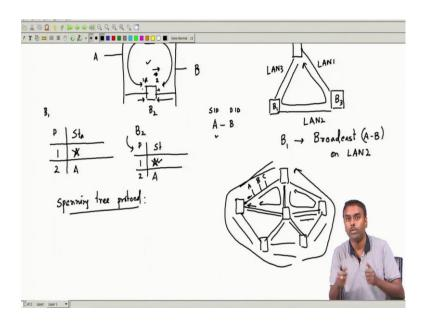
This is the protocol where if there are because of the topological design there are inherent loops. So, let us say I have these bridges they are connected like this ok? So, there are lots of loops as you can see these are all loops, the way bridges are connected there are multiple loops this bigger one also might be a loop.
