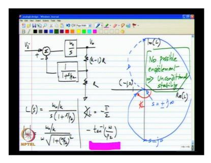
So, now let us take the next case where we have and in this case the loop gain L equals omega U by K S 1 plus S by p 2. And the magnitude of omega can be calculated to be omega U by K divided by omega and square root of 1 plus omega by P 2 square and the angle of L can be calculated to be minus pi by 2 because of this S minus tan inverse omega by P 2. Now, we can draw the Nyquist plot, the plot of imaginary plot of L versus real part L and we have this point minus 1, 0 as always.
