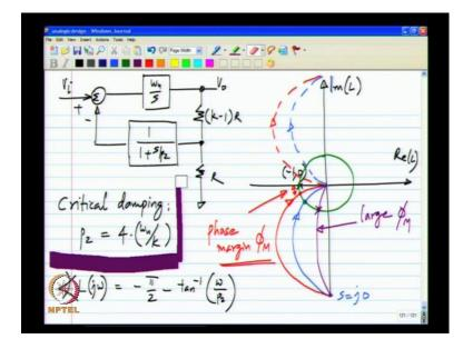
And our loop gain is known and the angle of the loop gain is minus pi by 2 minus tan inverse omega by P 2 it is minus pi at high frequencies. So, the Nyquist plot starts from minus infinity on the imaginary axis and this is minus 1, 0. And what happens is that it comes around like that asymptotically reaching an angle of minus pi. Now, it turns out that if you have a lower value of P 2 it does that a phase angle increases and it comes closer and closer to the negative real axis.
