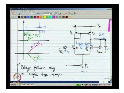
That is, the maximum rate of change of output, that is best illustrated by looking at circuit like this. Let us imagine that, the circuit has reached steady state with V bias at the input and V bias at the output. Now, let us say we apply a small step v i, some small value let me call it delta V, now what happens, the current in M 1 will increase by g m v i
