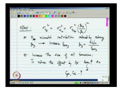
Let us quickly look at, how to optimize the offset and the noise, obviously the offset which is related to mismatch in the input differential pair and the load can be reduced by increasing the size of the transistors. So, first of all, the contribution from M 3 4 reduced by reducing g m 3, now let us say you want to reduce g m 3 alone and you do not want to
