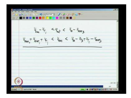
We also evaluated that, the output voltage has swing limits of, we decide 3 below V D D and at threshold voltage, below V bias and V bias itself has V bias plus V T 1 and a lower limit of V D sat 0 plus V D sat 1 plus V T 1. Both these ranges are skewed towards the upper side, they are lot closer to V D D than to ground and this is a consequence of using
