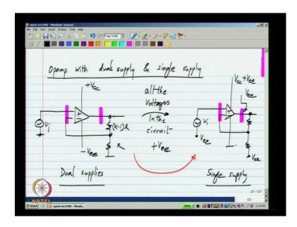
Now, normally when you see the text book introduction to the opamp, it will be operated with dual supplies and the input is just shown as, having a quotient value of 0, this is an example circuit. So, the quotient value of the output is also 0 and the quotient value of the input is 0, but this does not necessarily have to be the case, the quotient value of the input could be anywhere within the input common mode range of the circuit.
