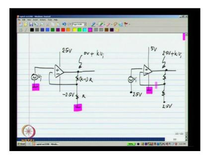
So, just to give an example, so let us have an opamp operating with plus and minus 2.5 volts, this is an non inverting amplifier of gain K. The output will have quotient value of 0 volts and on top of that, we will have K times V i, which is the incremental output, it will be K times the input increment. Now, exactly equivalent to this circuit is, if we have the opamp operating with the single 5 volt rail and v i terminated to 2.5 volts and this resistive divider also terminated to 2.5 volts.
