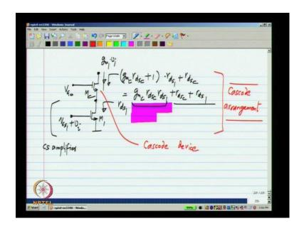
So, first let me discuss the output resistance of a single transistor, let us say it is biased with some voltage V g s 1, let me call this M 1. So, looking in here, I have resistance r d s 1 or a conductance g d s 1 and let us say, I use a common gate amplifier on top of this one. So, the lower one, I could think of as common source amplifier if I was going to
