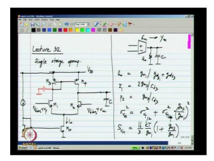
This is the tail current source and it will be biased from a current mirror, let us say that tailed current is I naught, this is the output and the output when loaded by capacitor becomes an integrator. Even if the capacitor is not expressively loading the output of the opamp, we will have the parasite capacitors, which will limit the unity again frequency. The drained parasitic of M 4 and M 2 will be part of the load capacitance or the integrating capacitance.
