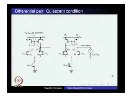
So, we said that this and that voltages are equal by symmetry. That is how we started the analysis. So, if we terminate Vd s plus Vg s 3, nothing will flow there and I naught by 2 flow through all these 4 transistors where I naught is the tail current.
