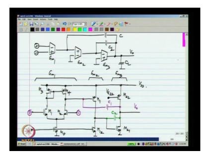
We know that at the signal level, what we need is three stages. This is the input of the opamp and that is the output. We can think of it as the input Gm 1, driving a current controlled voltage source with a transadmittance Sc and a transimpedance 1 by Sc and the current controlled voltage source is made this opamp ok?
