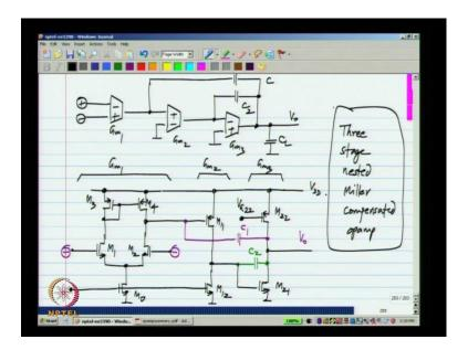
If you want to tailer to zeros in series with C 1 or C 2 or both, we can connect resistor in a 3 stage opamp. This is 3 stage nested Miller compensated Opamp. Let me copy over this circuit just illustrated the couple of details.
