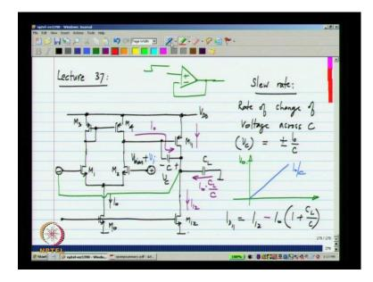
This is the second stage opamp, positive input, negative input and the output and this is integrated capacitor C. Now, we have to assume that there is some load here and the load will be connected between the output and ground. If it is the capacitor load; if it is a resister load we will see later what to do with it. We will assume that there is only a capacitor load for now. That is why the tile current of the input stage is I naught.
