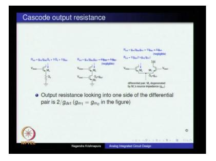
Now, the output resistance can be calculated using this. We know this is the output resistance of the cascade. It is given by this formula. When we have a resistor with conductance Gs and the source of the transistor Mc, we have another transistor. It will be Gd s 1 instead of Gs and finally, if we have a differential pair, it is as though this
