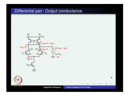
To calculate the output conductance, this is what happens if we apply a positive voltage Vt. We will have Vt of Gd s 1 by 2 flowing this way and that will also get an error. So, Vt of Gd s 1 by 2 will flow there plus Vt of Gd s 3.
