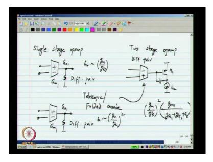
We have a single stage Opamp of some Gm 1 and this is just a differential pair. It has some G naught 1 and the DC gain approximately Gm by Gd s of a single transistor. We can also simplify this by going into telescopic or folded cascade. What that will do is to have a similar topology.
