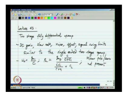
These all can be calculated for the fully differential case, but these will be similar to single handed two stage opamp. Now, the parasitic poles are also similar in that the unity gain frequency is g m 1 by C and the second pole is related to that. Except that, there will not be the mirror pole zero that is, the pole zero due to the current mirror is not present. Now, because of these reasons we would not discuss this further in perhaps a later
