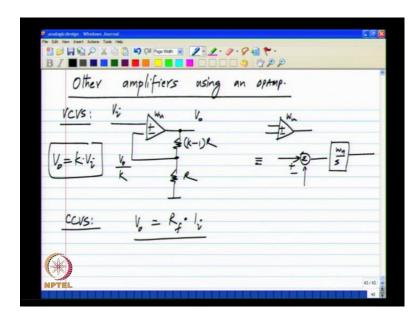
So, what we have so far is a voltage control, voltage source. Where, this stands for and omega u is an important parameter of the opamp. That will be given in the opamp data sheets and so on. So, in this case, what we did was, we took the difference between V i and V naught by k, integrated the difference to get the output. So, let us see, we want to make instant a current control voltage source.
