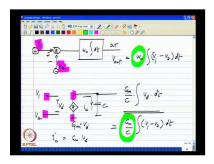
I will name this V 1 V 2 and I want to integrate the difference. This is my opamp, the plus and minus and the output terminals. So, if I choose to implement the integration with the capacitors, then this voltage will be 1 over C integral of i c d t, where i c is the current flowing through the capacitor. Now we would like i c to be related to the difference between V 1 and V 2. The way to do that is, to use a voltage control current source which I will show it as a symbol.
