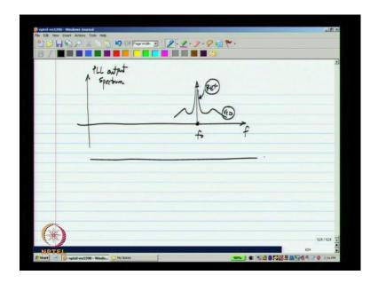
So, if you plug in any signal generator, which uses a PLL into a spectrum analyzer, it is very common to see a sharp peak corresponding to the periodic signal and phase noise, side bands like this were, here it is dominated by the V c o. And here it is dominated by the reference and of course, on the upper and lower side, you will have exactly the same things replicate. This by the way, is the spectrum of the voltage or current, which has this as the phase.
