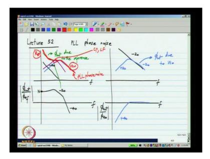
The phase noise of the reference oscillator will have 1 over f square frequency dependents that is, minus 20 dB per decade if you plotted verses frequency. And if you plot the magnitude of the transfer function from the phase of the reference signal to the phase of the output signal, that could be a low pass function, which would look somewhat like that. And the exact shape depends on the parameter chosen, but we except
