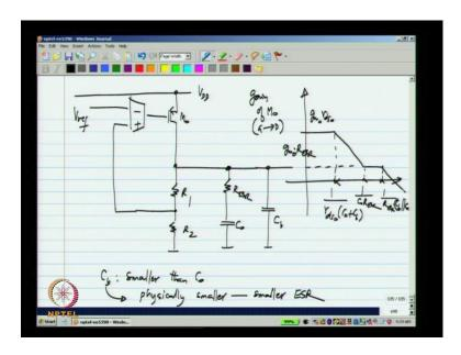
So, what is normally done is that we have the effective series resistance for this capacitor and to make sure that the effect of the effective series resistance is that high-frequency the impedance is does not reduce. So, what is V c done is to have another bypass capacitor, which is smaller much smaller than C0. So, C b physically smaller and has a smaller effective series resistance will assume that the effective series resistance of C b is negligible. So, this is what is usually done.
