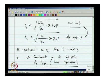
So, if I right it as a constraint on r o1 had to be smaller than square root of c g s0 by C0 in series with C b and g m1 g m0 times beta now, previously we had r o smaller than c g s0 divide by C0 and series with C b divided by c g s0 times that, where as a previously we had C0 by c g s0 times g m1 g m0 times beta now, C0 is much more than C b. So, the holder limit was greater than the new limit.
