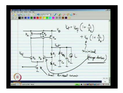
So, the simplest thing that we can do is the realize single stage op-amp this is biased with some current mirror and we apply V ref for their assuming that this is 1.2 volts there is enough rooms to accommodate this n-MOS differential pair otherwise you will have to use p-MOS, and then hold up the signals. So, this is the voltage regulator for efficiency you should use small quiescent current and also the output voltage here will be V ref
