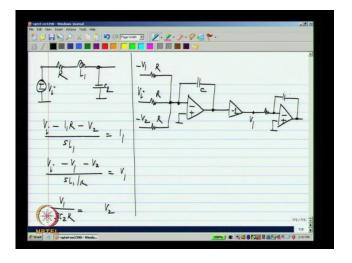
So, in this the first case we need to have an integrator with three inputs and this will be the output V1 under three inputs would be V i and minus V1 and minus V2, and the other integrator has also single input and that is equal to V1, I am running out of room here this would be V2 and I have to connect minus V2 over there, which appears over here.
