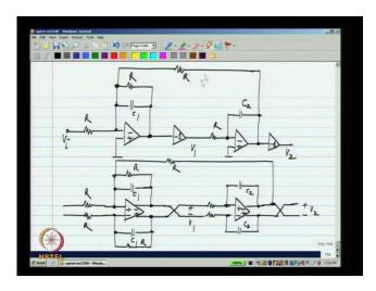
and feedback one for each side, and will have it to input resistors we are resistor cause each of these this minus one simply corresponds to crossing the wires like that even will have this capacitor and to get the actual output voltage V2 it will be simply to cross the wires, and V2 will be like that and V1 will be of that side finally, how to complete this feedback loop, which comes from minus V2 and the same on the other side.
