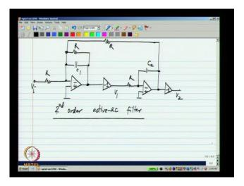
I will get topology, which is a classical active RC filter topology ((No Audio: 40:24 to 41:01)). So, the actual output must be inverted again to get rid of the polarity inversion, if I apply here I will get V1 and V2, where V1 is the scale version of the inductor current and V2 is the capacitor voltage in the prototype.
