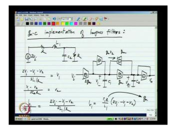
So, now, let us look at g m-c implementation of these low pass filters ((No Audio: 17:29 to 17:49)) will take the w terminated prototype(( No Audio:17:55 to 18:07)) and we know that this circuit is described by these two equations. So, in our active counterpart will have two capacitors C1 and C2, but voltages V1 and V2 across them, and V1 on V2 and the input Vi are related by this relationship. So, this part seems.
