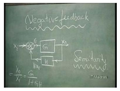
Negative feedback and its disadvantage was first mentioned in the form of reduction in forward transfer parameter. That is a disadvantage; but the advantage is the sensitivity improvement or reduction of active parameter sensitivity. This is called reduction of Active... What is it? Active parameter.
