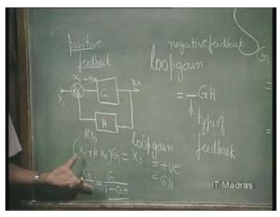
What is happening for the positive feedback? Unlike the negative feedback where the gain was always less than G, here the gain is what? - going to be greater than G. If G and
