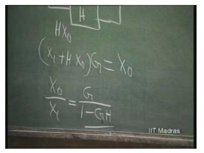
We are considering situations where G and H are both positive quantities. In such a situation, we can see that you have here G by 1 minus G H and the loop gain is...loop gain in this case is positive and is equal to G into H. So, this is for the negative feedback.
