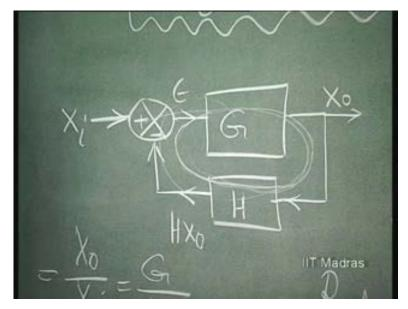
G into H is called the loop gain. This G into H...if the loop gain is very high, then obviously, 1 by 1 plus G H is going to be very very small. If loop gain is very high, then 1 by 1 plus this thing is going to be much less than 1.
