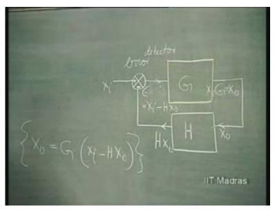
So, from this equation, X naught into 1 plus G H equals G times X i; or X naught by X i which is the important thing now, output divided by input in this basic feedback block, is always equal to G divided by one plus G H.
