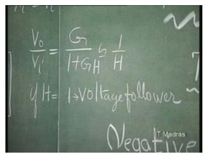
If complete output voltage is fed back without any attenuation at this point, this particular structure with H is equal to 1 is called a voltage follower. Once again, as far as error detector in this case is concerned, that can be done by what? - differencing the voltage, voltages. That is, input voltage is subtracted from part of the output voltage.
