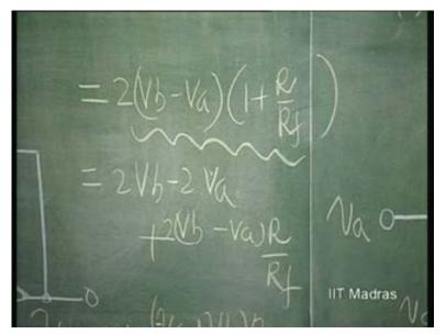
So, once again, we see that this is going to act as a differential amplifier, but uses only 2 op amps; and buffer stage...buffering action is still there because these are the non-inverting terminals here to which inputs are get...fed. So, these 2 instrumentation amplifier configurations are quite popularly used in practice.
