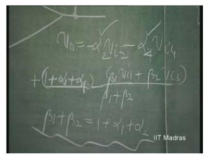
Then, I can conveniently select Beta 1 as V i 1 coefficient which is point 1 and Beta 2 as V i 3 co-efficient which is 100; so, this kind of design, can I do?
