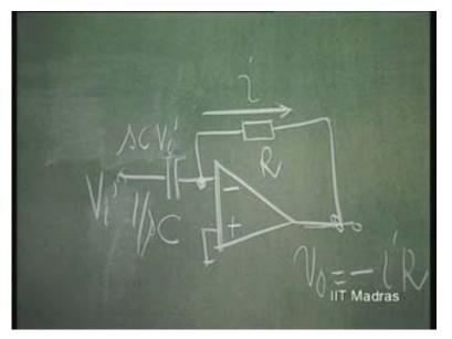
So, these are the transfer functions of these 2 blocks which are very important linear building blocks. What happens? Let us understand. For D C that is put S equal j Omega and consider for D C; Omega is equal to zero. The gain is infinity.
