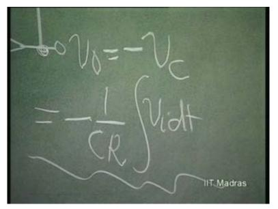
This is an important function, linear function, which is useful for a variety of applications in analog signal processing, integration. How we do differentiation? That is very simple. Once again, we have i equal to C d v by d t. That means, I have to establish a current which is proportional to an input voltage, let us say.
