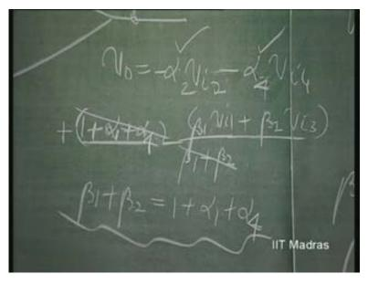
Beta 1 plus Beta 2. This is 1 plus Alpha 1 plus Alpha 4. This is equal to point 1 plus 100. 100 point 1. Which is greater? This is greater. Beta 1 plus Beta 2 is greater than 1 plus Alpha 1 plus Alpha 4 by an extent which is, let us see. That is all. 88 point 4. How do I give this? How do I therefore satisfy this?
