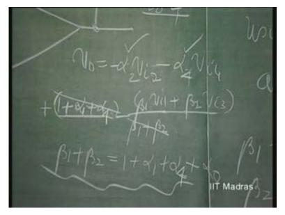
So, I simply put a resistance here with R... the input to this is zero; dummy resistance so that this generates an Alpha which is R by Alpha zero and Alpha zero is equal to 88 point 4. Now, this will have 1 plus Alpha zero; and we have purposely selected Alpha zero so that Beta 1 plus Beta 2 is equal to 1 plus Alpha 1 plus Alpha 2 plus Alpha 4 plus Alpha zero. They get cancelled here and we get this design in a very simple manner representing straightaway... Answer is very simple.
