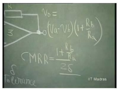
So, this circuit is one of the most popular circuits. It is available as an integrated circuit itself wherein two terminals have been brought out here so that this can be made variable if you want so as to vary the differential mode gain; and you can design it for any differential mode gain that you want. So, this circuit is one of the instrumentation amplifier set up.
