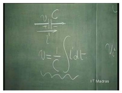
In fact, you can use this the other way about. C d v by d t is equal to I. So, it can be used either as an integrator, or integrator, or as a differentiator. The same capacitor can be used. How do we do it?
