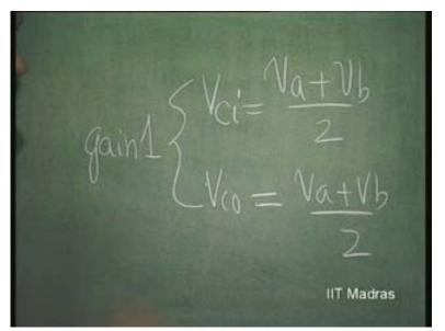
By introducing this stage, as far as the common mode voltage is concerned, the gain is just remaining 1. The common mode voltage input is V a plus V b by 2. Here also, it is V a plus V b by 2. But, as far as differential mode is concerned, here it is V a minus V b at the input; and here it is V a minus V b plus V a minus V b into 2 R b by 2 R a. These two will get added when we subtract it. So, this is equal to V a minus V b into 1 plus R b by R a.
