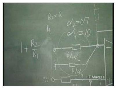
That means 1 plus R... R 1 is parallel combination of this, which is, Alpha 2 over R plus Alpha 4 over R. So essentially, you will get the gain as 1 plus Alpha 1 plus Alpha 2. Alpha 4; sorry.
