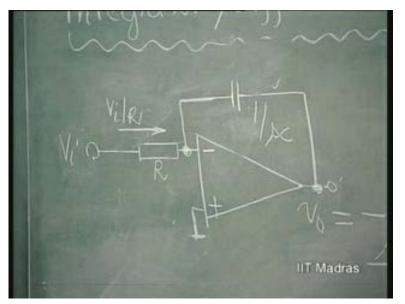
Next, integrator is something whose gain is inversely proportional to frequency. That means at high frequency, it eliminates all the signals; whereas differentiator is something that will amplify all high frequency components. That means a differentiator will respond even to noise which is occurring at high frequency.
