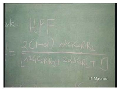
We can see that at very high frequencies, this S squared dominates. The output will be 2 into 1 minus Alpha. At very low frequencies, S equal to j Omega. Put Omega equal to zero. This is going to be zero. So, the output is going to be zero at zero frequency, goes to ultimately 2 into 1 minus Alpha at high frequency. So, it is called high pass filter.
