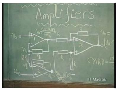
Common mode gain here, common mode voltage here, at the input is V a plus V b by 2. That is the common mode voltage at the input of these 2 amplifiers stage. At the output, again, V c i, V c o, here is again this; also equal to V a plus V b by 2 because these 2 get cancelled. So, the common mode voltage remains same. Gain is 1. (Refer Slide Time: 02:27)
