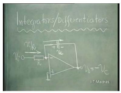
So, let us consider first, how integration is done or differentiation is done. Basically, operational amplifier is going to be primarily used to convert voltage to current. What is done is...integration or differentiation can be done by using a capacitor or an inductor.
