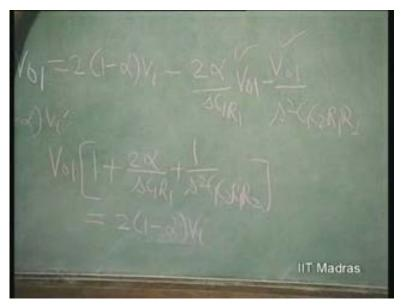
Or, V naught 1 over V i which is called the transfer function. V naught 1 over V i is equal to 2 into 1 minus Alpha divided by S squared C 1 C 2 R 1 R 2 plus 2 Alpha S C 2 R 2 plus 1 into S squared C 1 C 2 R 1 R 2. From the equation here, this is what we get.
