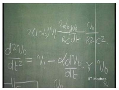
So, we can see here that essentially I have got the right hand column on this side with the proper sign except that these co-efficients have to be properly selected in order to make whatever they are. This may be made equal to 1 and this is 2 Alpha naught by R C is made equal to Alpha; and Gamma is equal to 1 over R square C square; like that you can select.
