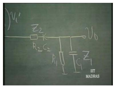
So, output V naught is going to be 1 plus R b by R a times V i, which is the input to be Z network, into Z 1 by Z 1 plus Z 2; or, this is also equal to 1 plus R b by R a into V i; dividing by Z 1; 1 plus Z 2 into Y 1. So, this is equal to 1 plus R b by R a into V i...1 plus Z 2 is R 2 plus 1 over S C 2; R 2 plus 1 over S C 2. Y 1 is 1 over R 1 plus S C 1; 1 over R 1 plus S C 1.
