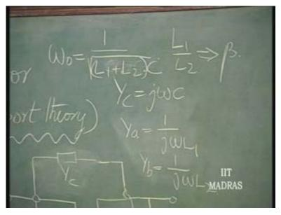
This can be determined by replacing Y c by j Omega C, Y a by 1 over j Omega L 1, 2 Y b by 1 over j Omega L 2. So, please work this out as a problem. So, let me now give you the complete problem.
