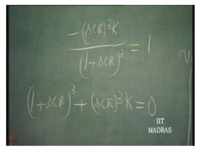
This cubic equation 1 plus 3 S C R squared plus 3 S C R plus S C R whole cube will come out of this, plus K. So, K plus 1 into this should be equal to zero. Now put S is equal to j Omega. So, we get 1 minus 3 Omega squared C squared R square plus 3 j Omega C R plus... That is actually minus, j S cube C cube R cube. One j square will give you minus and another j will remain K plus 1.
