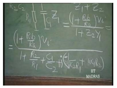
That means it will be in phase; output will be in phase with the input at that frequency. So, this quantity is the one which contributes to phase shift. So, that happens equal to zero when Omega naught is equal to 1 over root of C 1 C 2 R 1 R 2. That is the frequency of oscillation.
