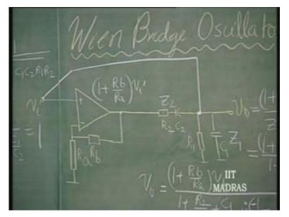
So, the condition for oscillation is that R b by R a has to be made equal to R 2 by R 1 equal to C 1 over C 2. This is easily done by setting R 2 equal to R 1, C 1 equal to C 2. R b by R a has to be then equal to 2. So, if R 2 equals R 1 equals R, C 2 equals C 1 equals C, then the frequency of oscillation Omega naught is 1 over R C; and the condition for oscillation is that this is equal to 2.
