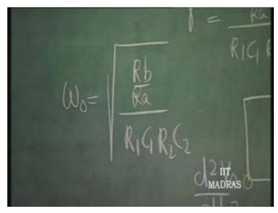
Now, if therefore output can become equal to input in magnitude...by connecting this, if I break the loop and then at a certain frequency if output can become equal to input in magnitude and have zero phase, then I can close the loop and make an oscillator out of it; or, if the loop gain, the loop gain becomes equal to 1 at Omega naught, only at Omega naught, then it becomes a sine wave oscillator at Omega naught.
