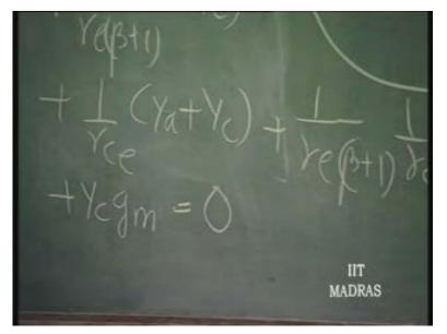
Now, when such a condition is to be satisfied, we have to see that it is possible. What does it mean? This will obviously have real part and imaginary part and this should be possible to make the real part go to zero and imaginary part also go to zero. Now, that can be done by selecting one possible combination - Y c as being equal to 1 over j Omega L and Y a equal to, let us say, j Omega C 1 and Y b as j Omega C 2.
