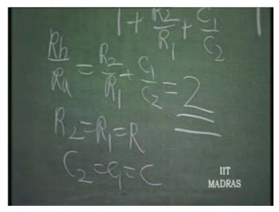
Now let us consider another oscillator. Once again, I am going to break the loop here. Let us assume that this loop is broken here. This resistance of R is going to really appear as resistance to ground here; this much of ground. So, in effect, this loading effect of the input resistance of the amplifier is coming here as R. So, actually speaking, so V i is going to be developed there.
