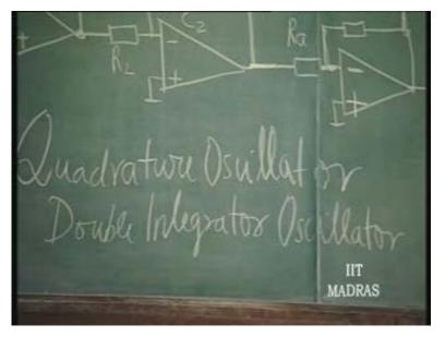
Quadrature because if this is V t sine Omega t, this will be V t cos Omega t. V t dash cos Omega t; and therefore, frequency of oscillation, Omega naught in this case, is root of R b by R a R 1 C 1 R 2 C 2.
