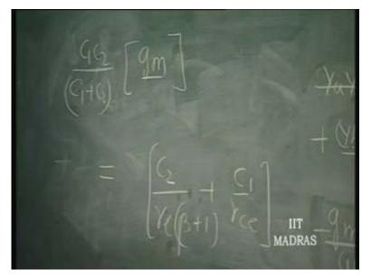
Essentially, this can be ignored compared to this, normally. Or, you can take that also into consideration. So, g m into C 1 by C 1 plus C 2 - this is the condition to be satisfied. Now, g m can be taken...g m into r e is very nearly 1. g m is equal to 1 over r e. So, this divided by g m into r c e. So, 1 over Beta plus 1 should be equal to C 1 by C 1 plus C 2.
