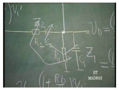
This ganging becomes necessary because R 2 by R 1 plus C 1 by C 2 should be equal to 1; R 2 by R 1 C 1 by C 2, both should be equal to 1 and total should be equal to 2; so the ganging becomes necessary.
