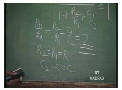
So, if it is greater than 2, R b by R a is greater than 2, it will start building up oscillation. Gain is greater than 2. If it is less than 2, it will start decaying. If it is exactly at 2, it is having poles on the imaginary axis. This system with this kind of feedback will have poles on the imaginary axis. So, this is an oscillator.
