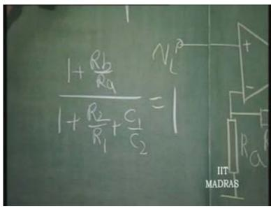
So, I can now connect the output to the input. It will oscillate at Omega naught equal to 1 over root of C 1 C 2 R 1 R 2.
