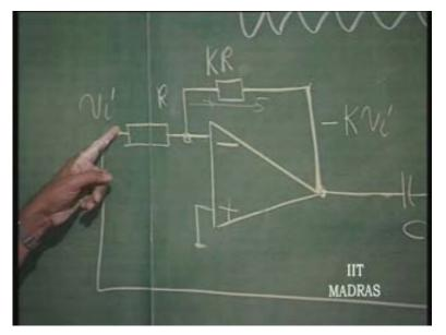
So, we have got a 180 degree phase shift which is independent of frequency here. In order to make it now come in phase, we have to provide additional phase shift of 180 degrees. That is why this is called phase shift oscillator. Additional phase shift can be offered by three such R C networks, in order to prevent this from loading. Otherwise, I might have to use a higher gain amplifier here. I am using buffer stages. This is only illustrating the principle of phase shift oscillator.
