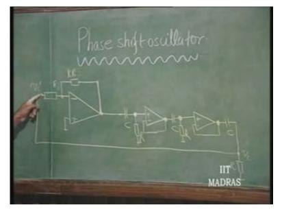
We have to see whether V naught developed here is same as V i. So, if V...this is V i; this is minus K times V i. This we have seen. As an inverting amplifier, if this is V i, this is ground; this is virtual ground. Current in this is V i by R; the same current will flow through this and develop the potential here, which is negative; and minus K times V i is the output here.
