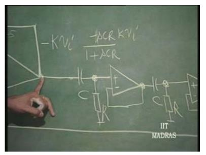
So, I put two such networks. So, we get here minus S squared C squared R squared divided by 1 plus S C R whole square, the gain; into K times V i here; and at...that is at this point also, it is going to be the same because of the buffer.
