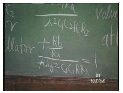
So the loop gain...that is, now I can close the loop and it will act as an oscillator. So, this is another way of looking at the oscillator.
