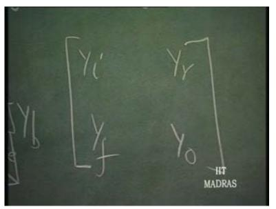
In such a situation, what is the loop gain? We have seen that Y f Y r divided by Y i Y naught is the loop gain; Y f Y r divided by Y i Y naught is the loop gain; and that loop gain has to be made equal to 1; or 1 minus Y f Y r divided by Y i Y naught should be equal to zero; or Y i Y naught minus Y f Y r should become equal to zero, Assuming that Y i and Y n naught do not go to zero at any frequency.
