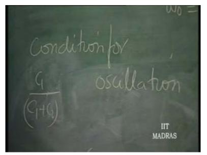
If r c e is infinity, then this also goes. The frequency of oscillation becomes exactly this. The condition for oscillation becomes very simple. Beta plus 1 becomes equal to 1 plus C 2 over C 1. So, 1, 1 get cancelled. So, Beta becomes equal to C 2 over C 1. Or, C 2 over C 1 has to be chosen to be equal to Beta. That is the condition for oscillation.
