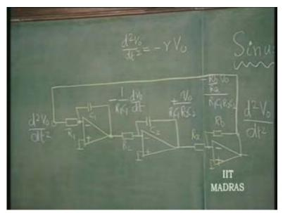
So, we can connect this; and this connection will make d square V naught by d t square equal to minus Gamma V naught, where Gamma according to us is nothing but R b by R a divided by R 1 C 1 R 2 C 2. This is also called Omega naught square, the frequency of oscillation being Omega naught; root Gamma is the frequency of oscillation.
