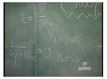
That means two of them are capacitive and one is inductive; or, this is in a capacitive and the other two are inductive. The feedback element should be of one type and the other two should be of the opposite type. So, that way, we will see that we have two types of oscillators. One - Y c is inductive, Y a and Y b are capacitive; another - Y c is capacitive, Y a and Y b are inductive.
