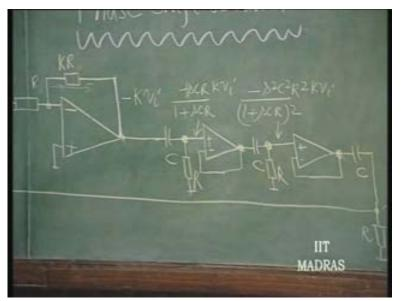
This is a phase shift oscillator. Again, you can have the phase shift as being brought about by R here, C here, R here, C here, all that. That will bring about, instead of this, root 3 divided by C R; and the K is going to be same as 8.
