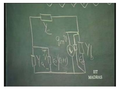
So, this is, let us say, input port; this is output port; this is the feedback. So, in a two port theory, how do I make sure that the loop gain is equal to 1 at a certain frequency? Loop gain, when it comes to loop gain, we saw that if I write down the matrix of the entire parameter... now I consider this a Y parameter and I have Y i here Y naught here.
