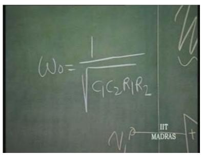
At that...when this is becoming equal to zero, the attenuation is 1 plus R b by R a divided by 1 plus R 2 over R 1 C 1 over C 2. If this becomes equal to 1, then output is equal to input and it is in phase.
