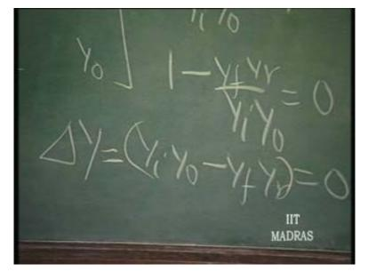
That means what is this? This is nothing but capital Delta Y. So, the condition for any oscillator according to two port theory is that the Delta Y should go to zero at Omega equal to Omega naught; a single frequency.
