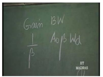
Gain into bandwidth is constant, which is equal to Omega d into A naught. This is invariably true. If you use this amplifier in any negative feedback configuration like this, gain into bandwidth remains always a constant.
