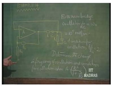
Now determine the change in frequency of oscillation and condition for oscillation when A becomes, not infinity as it was assumed here; A is finite and frequency dependent; 10 to power 6 by 1 plus S by 10.
