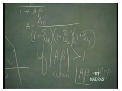
What is it? The loop gain in a negative feedback system... when the... when the phase shift of the loop gain becomes equal to 180 degrees, the magnitude of loop gain should be less than 1. Then only it is a stable system.
