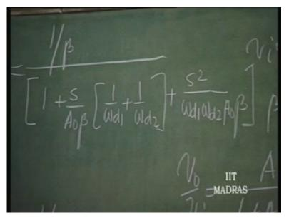
Once again, you expand this and this is 1 over Beta which is the gain of the amplifier with feedback, plus 1. We will ignore 1 over A naught Beta compared to 1; and then you have S into A naught Beta, 1 over Omega d 1 plus 1 over Omega d 2; plus S square into Omega d 1 Omega d 2 into A naught Beta.
