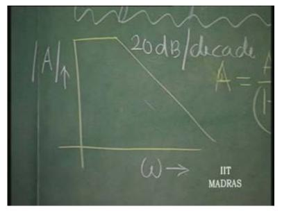
We have seen that gain becomes A by 1 plus A Beta, let us say, for a voltage control voltage source with H feedback, because that is what it... what makes the voltage control voltage source go towards its idealization, H feedback; and this is Beta. This is corresponding to R 1, let us say R a, this is R b. Beta is equal to R a by R a plus R b. All these things, we have earlier understood.
