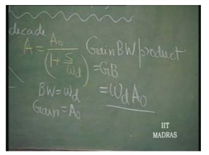
Just look at it. Come to this. Amplifier with feedback. This is the feedback gain. What is the gain? 1 over Beta; gain is 1 over Beta; and its bandwidth is A naught Beta into Omega d.
