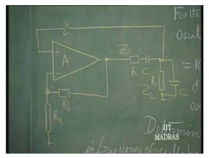
Z 2 by Z 1 plus Z 2 which is therefore the loop gain. I will close this loop. That means this is going to be made equal to 1. So, that is the condition for making this go into oscillation.
