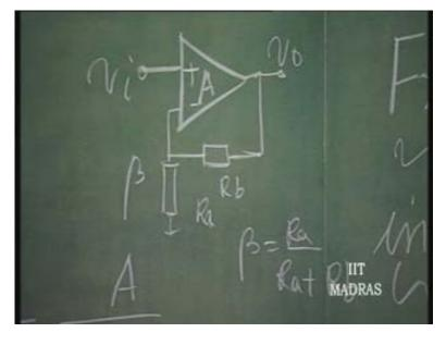
So, the gain V naught over V i is going to be... this also we have derived earlier. So, dividing by A Beta throughout, this is 1 over Beta which is the ideal gain divided by 1 plus 1 over loop gain. This is important. The error is always 1 over 1 plus 1 by loop gain.
