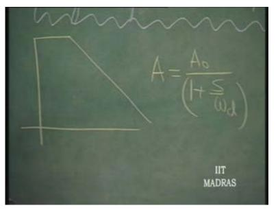
I am considering this as Omega d because this is supposed to be the only dominant pole in the entire amplifier in its useful frequency range. That is why I call it Omega d. A naught is the D C gain at S is equal to j Omega, Omega equal to zero; and it is going to fall off at let us say, 20 decibels per decade.
