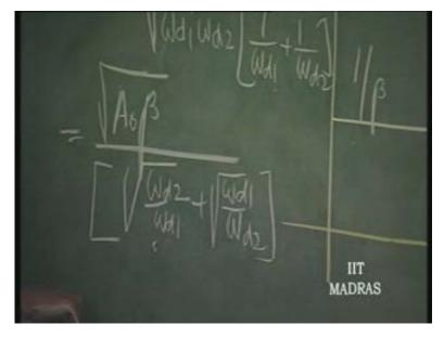
This is something like x plus 1 over x and that is going to be maximum, if you want, when x is equal to 1; and this value can contribute to half only. At therefore Q of this system is directly proportional to root of A naught Beta. If the loop gain is high therefore,
