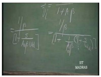
Let us consider. We started with an amplifier whose gain was A naught and this is called the bandwidth. Omega d is then the bandwidth. The point at which the gain falls to 1 over root 2 times the maximum; or, it is also called minus 3 d b point. The gain falls to 1 over root 2. So, this is the bandwidth. The gain of the open loop amplifier is A naught.
