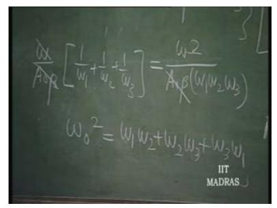
This is the frequency at which the phase shift becomes equal to 180 degree and at that point, the amplifier with feedback will have a gain going to infinity. How does it become infinity?
