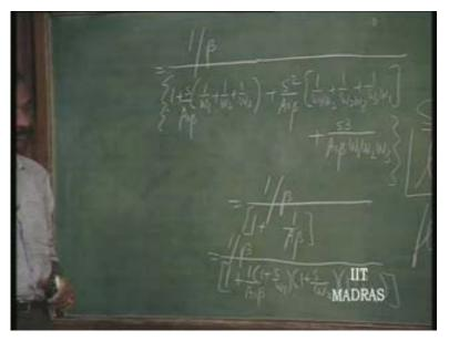
What is the problem? The problem is if you put S is equal to j Omega, S is equal j Omega, then this becomes Omega squared. This becomes minus j Omega cube. So, you can see here, it was originally having no phase shift. Now, it can have a phase shift of 180 degrees. That is the loop gain. Then what happens if it has a phase shift of 180 degrees? Then it becomes purely real.
