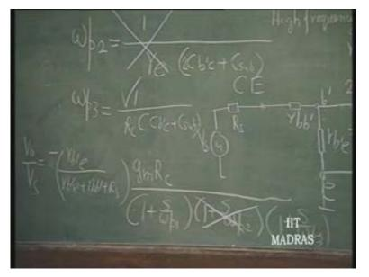
And, it is really speaking, a 2 pole system even now because this pole, intermediate pole, is at very high frequency at which point the gain might have fallen off to less than 1. So this, because of Omega p 1 and Omega p 3, the gain fall off occurs. Which one is the one that is going to determine the cut-off frequency really now depends upon the magnitude of the source impedance as well as the magnitude of collector resistance.
