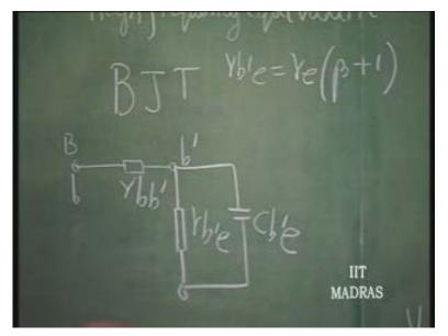
So, we have the emitter here. Then, from the base to the collector, there is a capacitance because it is a reverse biased junction. So, this is c b dash c. This is going to be lower in order because this is a forward biased junction. This capacitance is called diffusion capacitance. This is going to be pretty high compared to c b dash c.
