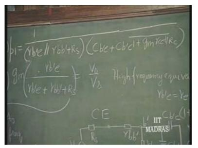
That can be written by observation. Always find out the net capacitance and the net resistance across the capacitance. That will determine the time constant at any point. So, C b dash e plus C b dash c into 1 plus g m r c e parallel R c is the net capacitance. Across that capacitance, we have a resistance of r b dash e parallel r b b dash plus R s.
