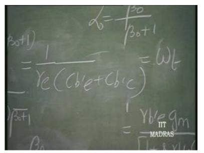
f t is Omega t divided by 2 pi. So, this is called transition frequency. What is transit? The gain actually, after this frequency, becomes less than 1. That is, Beta, if you consider, Beta itself is going to fall to magnitude which is less than 1.
