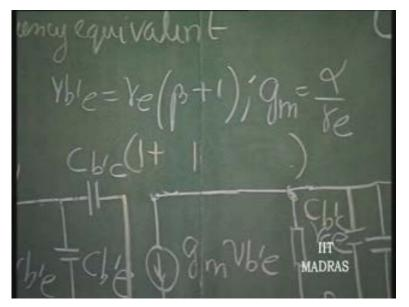
And by the same token, this this C b dash c will be 1 plus 1, that is 2. That is an increase here because there, the gain is now not negligible. So, the output voltage and input voltage, they are of the same magnitude, but opposite in phase. So, we get 2 C b dash c here at the output and 2 C b dash c at the input. Is this clear? So, 2 C b dash c, 2 C b dash c there.
