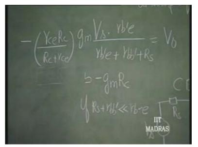
When we are using a voltage source drive, the gain of the amplifier and then r c e is much greater than R c. This is the normal gain of a common emitter amplifier.
