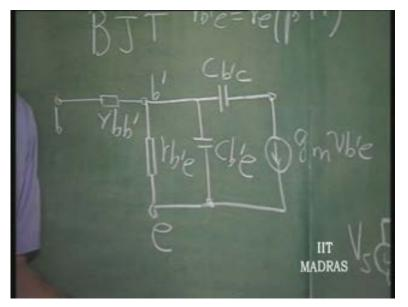
So then, actually, g m is Alpha divided by r e according to us; low frequency. That is going to give you the low frequency collector current; and across the collector we have the so called r c e. That current source is not ideal current source. There is a shunt resistance r c e typically of the order of few mega ohms, in the case of integrator circuit transistors. So, this is what is called hybrid.
