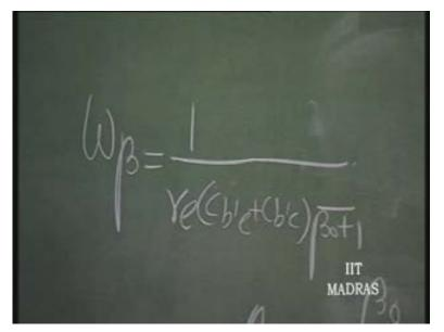
Let us now see what is Alpha? Alpha at high frequency is nothing but Beta at high frequency divided by Beta plus 1. This we have always known. So, this is equal to, let us write it as, let us say, 1 by 1 plus 1 over Beta. 1 over Beta here can be substituted from this as 1 plus S by Omega Beta divided by Beta naught.
