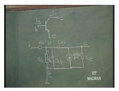
This is the common emitter transistor. This is the hybrid pi equivalent. So, at low frequencies, these capacitors are not coming into picture. So, I know that I short circuit this, then I c by I b is called Beta by definition; is called short circuit current gain of a common emitter transistor. That means this is shorted.
