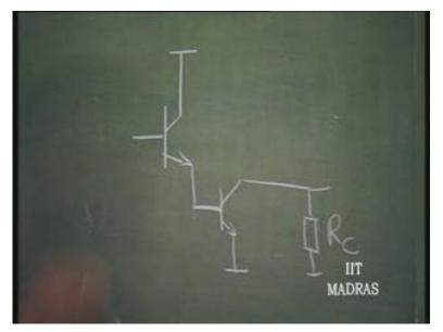
Here, I am putting... if R s is pretty high, let us say; R s is not very low. If I directly connect R s, R s parallel r b dash e is going to be shunting the capacitor. If I put it through a common collector stage, then this is still r b dash e parallel... Now, r e plus R s into 1 minus Alpha is the impedance that is shunting this.
