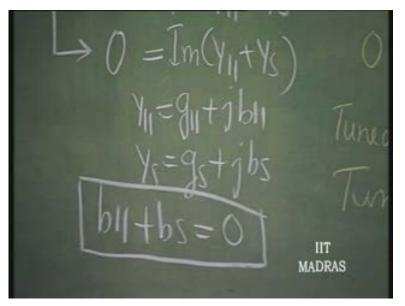
The susceptance of the input device plus the susceptance of the source is made equal to zero. If this is capacitive, then obviously this has to be inductive in order to make this equal to zero. So, this is what is meant by tuning. In such a situation, the entire Y i total is going to be twice g 1 1 because g s is made equal to g 1 1. This is called matching.
