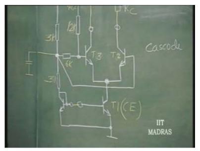
So, this is signal wise grounded by means of a capacitor. This is connected to V C C and we see that if A G C terminal is left free, there is almost no current through c k...6 k and the base of this T 2 is at the same potential as the base of T 3; and therefore, these two currents will be very nearly one and the same.
