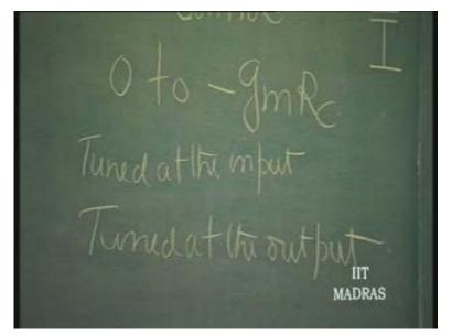
Now, let us understand what is meant by tuning. Let us say, the input impedance of cascode structure Y i is equal to Y 1 1 because Y 1 2 is zero; because Y 1 2 is zero. Because Y 1 2 is zero, there is no interaction between output tuned circuit and input tuned circuit. Otherwise, it will be very difficult for us to tune the input, independent of the output. Output and input will start interacting with one other, one another because Y 1 2 is zero.
