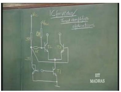
So, how do we get a cascode connection in this is what we are going to discuss. So, T 1 is actually the amplifier which is connected as common emitter here; and we will make this T 2 so that this is the common base amplifier. So, this combination - T 1 and T 2 can be used as a cascode. If, for example, I connect externally externally I connect V C C C to this so that this transistor may not come into picture in the actual structure and here I
