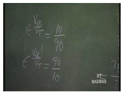
So, if this is divided by the... one is divided by the other, we get V 6 K minus V 6 K prime by V T as being equal to 81; or V 6 K minus V 6 K prime is equal to V T log 81, which is equal to...1 naught...109 point 86 millivolts. So, you can see that if I am to control the voltage here, the change in voltage necessary at the basis is about 110 millivolts; approximately equal to 110 millivolts. V 6 K prime minus V 6 K is equal to 110 millivolts. So, this is... this is the change that...
