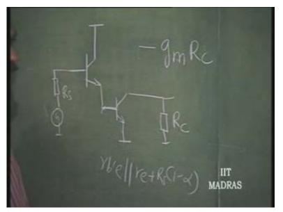
So, for these two things, the gain is remaining the same as common emitter. Here, it is halved. So, this also is wideband pair. All these three wideband pairs can be used for high frequency application of video amplifiers.
