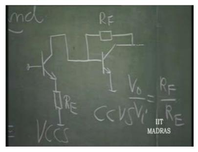
So, I would just want to indicate that for biasing purposes, you have to put a resistance from here and a resistance from here to V C C. So, this is R c 2, this is R c 1; and I just want to indicate how this can be converted into an I C without using capacitors, by pass capacitors, etcetera. So, let us convert this.
