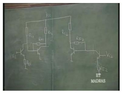
Then I want to convert this into an integrated circuit. The basic principle is whenever you have a symmetric structure like this, the ground, this is the common point, can be lifted; and you can make it go through a current source I naught a, I naught b, minus V E E and plus V C C. So, this becomes a wideband I C.
