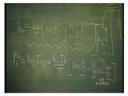
Now, we would like to find out the power dissipated during that time. You look at it. This is the time during which there is a current pulse by the transistor. This is the time during which the transistor is conducting. Now we can clearly say that when it is not conducting, the potential here is going to be V c c. This is a coil here. So, the potential here is going to be V c c. No current is there.
