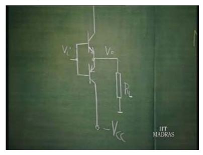
Now, how to get rid of cross over distortion using negative feedback? Use an op amp as a driver stage for this output stage and then connect the op amp in its negative feedback configuration. So, this can be connected in negative feedback configuration either by using inverting stage or a non-inverting stage. Now I am going to do it by using an inverting stage, negative.
