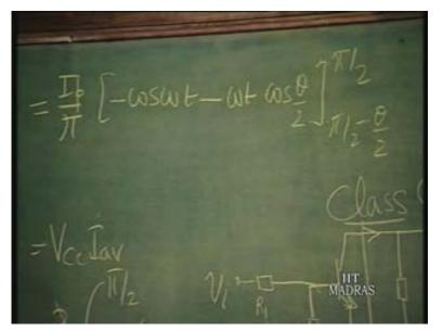
So, this is equal to I p by pi, minus  $\cos pi$  by 2 is zero, minus pi by 2  $\cos$  Theta by 2. Then the other limit which is minus, minus this. So here, it will become plus. Both will become plus. And therefore, plus  $\cos Omega t - \cos pi$  by 2 minus Theta by 2 which is sine Theta by 2;  $\cos pi$  by 2 minus Theta by 2 which is sine Theta by 2. That is over; plus pi by 2 minus Theta by 2 cos Theta by 2.
