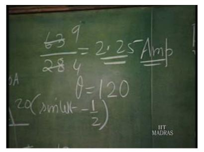
So, this completes... in sense, the complete design of the output stage of our transistor, power amplifier. Input stage - please remember. You have to now design this value of V B B and this value of V i R 1 R 2 in such a manner that this kind of current wave form is coming.
