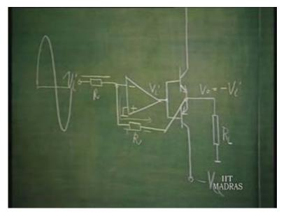
Now, let us see what happens really if the diodes do not conduct. When this voltage is zero, obviously, these diodes do not conduct. When the diodes do not conduct, there is no feedback from this. This, we will call it as V i dash now. There is no feedback from the output of the op amp to the input. If there is no feedback, this is under open loop.
