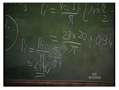
That means actually, power dissipated, which is also an important thing in the transistor, is going to be 63 watts minus 56 watts which is going to be about 7 watts.
