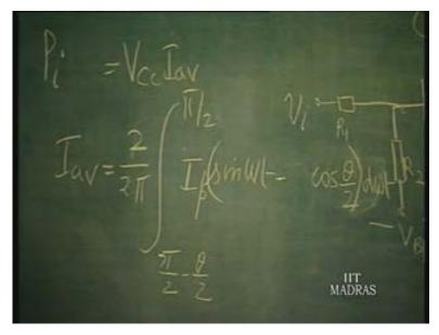
So, this is nothing but I p by pi. This I p divided by pi into integral of sine Omega t is minus cos Omega t minus Omega t cos Theta by 2; the limit from, let us say, pi by 2... minus Theta by 2 to pi by 2. So, this is the average.
