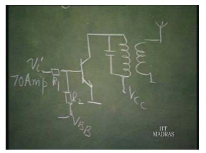
So, let us now see the design. How this is going to work. I max is chosen from this I c max, the collector current, 16 amperes. So, we will... let us select something like 10 amperes as the permissible maximum current we will have for the transistor, typical operation.
