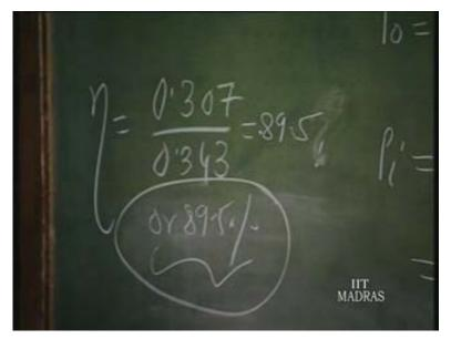
In the design, output power is 56 volts; efficiency is nearly 90 percent. That is, 10 percent of the power is only wasted in the device. So, once you have this efficiency, the input power is going to be output power divided by the efficiency. So, which is very nearly 56 watts divided by point 9. I am approximating point 895 as point 9. This is... how much? About 63 watts? Yes, 63 watts. Pardon? Yes. So, 63 watts is the input power.
