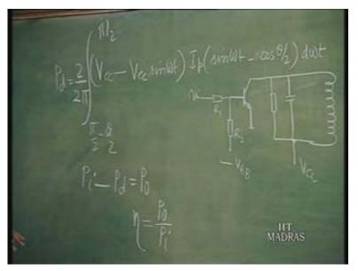
So, if you work out this integral, it will come out to be V c c I p by pi into sine Theta by 2 minus Theta by 2 cos Theta by 2 plus sine Theta by 4 minus Theta by 4. So, this is the power dissipated in the transistor; average power dissipated in the transistor. So, this will be very helpful for you to find out what the transistor rating should be.
