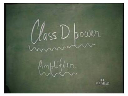
So, let us now discuss what is meant by Class D as against Class A, B, C. Class A - the situation was this; that the amplifier was kept in readiness to receive the signal. So, it was working continuously. Whether signal was there or not, the amplifier was dissipating considerable amount of power. When the signal appeared, the power that is dissipated in the active device gets converted into useful signal power. With this resultant defect, it became an inefficient scheme.
