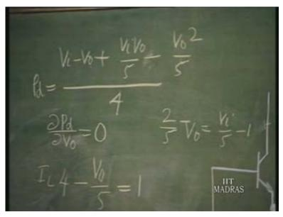
Now, we want this equation...of this condition to be satisfied at a specific value of V naught. What is the value of V i? So, this is going to be satisfied at V naught equal to 15 volts, 15 volts, if V i by 5 is equal to this. That means 6 plus 1 - 7 for V i equal to 35 volts.
