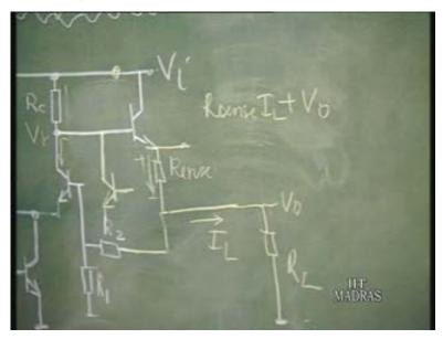
So, I take only a portion of that voltage. Let us put this as R a and R b, an attenuator. We will therefore put it, put this as R into Alpha; R into 1 minus Alpha. These are two resistances. What matters is the ratio.
