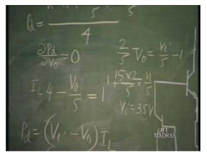
So, for V i equal to 35 volts, this is going to be satisfied. That at V naught equal to, in this line, at V naught equal to 15; that is where we want. We could have located it here or here or here. We want purposely, this to take place here. If you want it to locate here, V i should have been still higher. So, for V i equal to 35 volts, this gets satisfied and we can find out the power dissipation maximum there, from this expression here.
