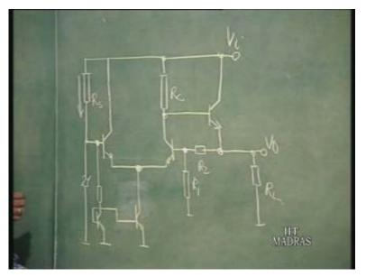
How to improve line regulation? This also influences in what is called ripple rejection because as ripple will appear at V i and that V i will cause change in current in this, that will cause a change in voltage normally; and that change in voltage will also come as 1 plus R 2 over R 1 at the output. So, both ripple rejection and line regulation factor can be improved if we make the current here constant. One way is to put a current source.
