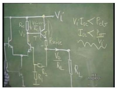
It can be low compared to load resistance. So, the output resistance is kept low. So, this sense resistance will sense the load current here. So, what is the load current? V naught by R L. So, this V naught by R L will flow through the sense resistance and if R L is decreased, this current increases and this voltage increases.
