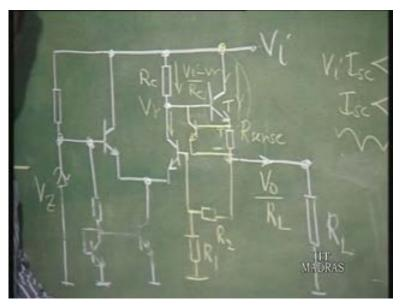
So we have this protection transistor getting forward biased because of the current that is flowing through R sense; and when I into R sense, when this becomes equal to V Gamma, the cut-in voltage of the transistor, this transistor starts conducting.
