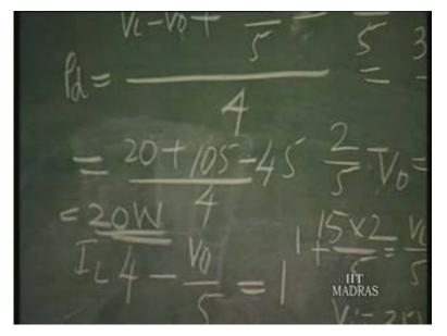
That means, if that happens, the maximum power dissipated at this knee is going to be 20 watts. That means the transistor that I had to select, its rating should be greater than 20 watts. So, this is an important criteria for the design.
