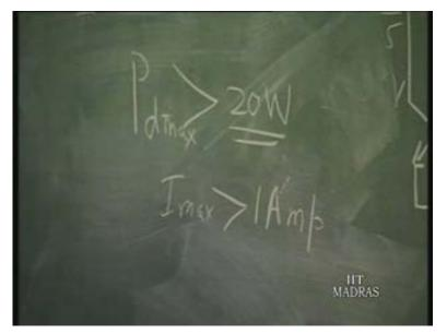
These are the important ratings for the power transistor. That is the pass transistor. So, you will see that this has resulted in a considerable amount of drop in the so-called this resistor. See... Let us now find out. This is 15 volts; and when the current is 1 ampere, there will be a drop of 5 volts here.
