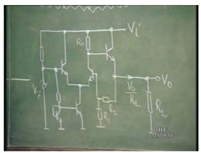
It is the external circuit that is put so that this is V z into 1 plus R 2 by R 1. This is the regulated voltage at which it is maintained. Up to what current can it maintain this? This also we had discussed in terms of the ability of this circuit to function.
