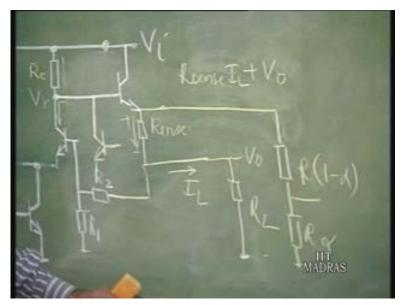
So, the voltage appearing here is going to be this whole thing. This is the voltage here. That into Alpha; that will appear here. Alpha R by Alpha R plus R into 1 minus Alpha which is R itself. So, Alpha... So, the voltage here is Alpha times this. This is the voltage here. That also may be too high a value, minus V naught. So now, I have two ways of making the voltage pretty small. Alpha is chosen such that this large voltage is set to a small value, and I subtract V naught.
