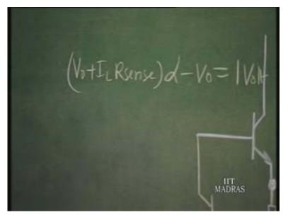
When V naught is zero, the I Hold is point 25. So, I L is point 2 5. R sense to be found out, into Alpha; this is equal to 1 volt. So, R sense into Alpha is equal to 4 ohms. 1 by point 25 which is 4 ohms. This is determined from this hold current.
