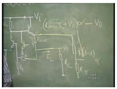
That is because between base and emitter, you are applying some potentials of the protective transistor, transistor which is coming to protect this whole thing. So, if I connect it that way now... So, what is the way? This base is connected to this point. This way. Let us therefore connect it there and emitter is connected to V naught. So, the base potential is this.
