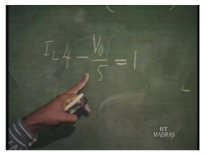
Therefore, suppose I L and V naught vary in this line. Then, what is the dissipation maximum, power dissipation maximum in my transistor, which is getting V i minus V naught as its voltage and I L as the current? So, V i minus V naught as its voltage and I L as the current? Ne would like to maximize this and set the limit at I knee for a specific value of this.
