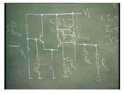
Now, let us see the protection we have rendered for this transistor, pass transistor. At what cost, let us examine it. See, after all, it is not that every day I short circuit the voltage regulator. That is normally an accidental thing.
