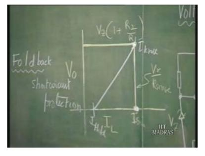
But now, I knee can be much higher for the same rating of the transistor; then I short circuit because now, we can examine that the power dissipated is going to be lower. Particularly under short circuit situation, it will be pretty low. So, until the short circuit is removed, it can remain in this. So, no harm; particularly in regulators which are not likely to remain attended for long periods of time, this kind of short circuit when it occurs, it might destroy otherwise, the regulators.
