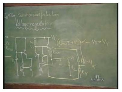
So, we can apply the limits to these two points and we get the equation of the line. So, if that is the case, then you can now see the two variables R sense and Alpha. Why two variables are necessary here? Because it has to go through two points here.
