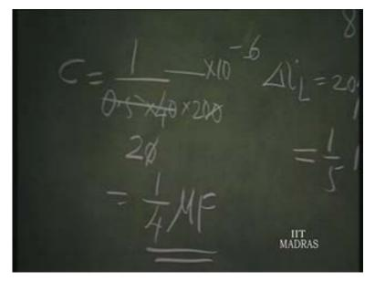
So, if you use a capacitor here which is point 25 microfarad, this should be good high frequency capacitor because this switching frequency is 200 Kilohertz. Please remember that. So, you have to use a good high frequency capacitor here. Point good quality capacitor with very low series resistance, etcetera. Capacitor is already determined.
