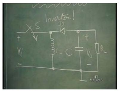
So, this in fact is the most popular circuit for switched board regulators primarily because here there is no restriction on the fact that output voltage has to be always less then input voltage or output voltage can only be more than the input voltage, or anything. Output voltage can be anything in relation to input voltage. That means it can do both boosting and at...what is that? – reducing.
