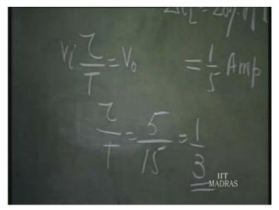
So, tau over T is equal to 1 over 3. Now, using this information, we can actually find out the inductor because inductor value is, strictly speaking, the voltage across the inductor is going to fall at this rate; V naught over L into T minus tau. V naught over L into T minus tau or V i minus V naught; this also is equal to V i minus V naught over L into tau.
