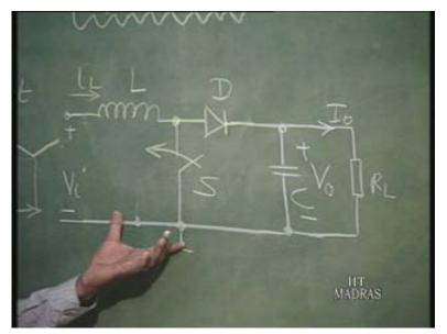
We have seen down conversion, then up conversion. We would like to now have an arrangement where it can be inverted. What I mean is with reference to a common point, reference...we have let us say, plus 5; only plus 5. We would like to get minus 5. This will be the situation when we are dealing with, let us say a logic circuit supply which is only, let us say plus 5. But, we would like to generate both plus 5 and minus 5 for making our analog circuits work; dual supply.
