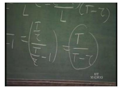
So, this is always higher than T minus tau. So, V naught is always higher than V i. So, this is called up converter. So, basic principle remains the same except that position of all these elements have got changed.
