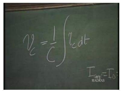
That means integral of the current waveform, changing current waveform...changing current waveform is what is marked in the...as a triangular waveform here. This average is removed. Then this is the changing current waveform riding over this. This current alone flows into the capacitor, we will assume.
