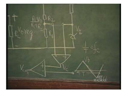
So, for what time it is going to be controlled, etcetera, is going to be decided by this switch here. So, this output of the output level here will be such that it is closed or open depending upon the duty cycle period here.
