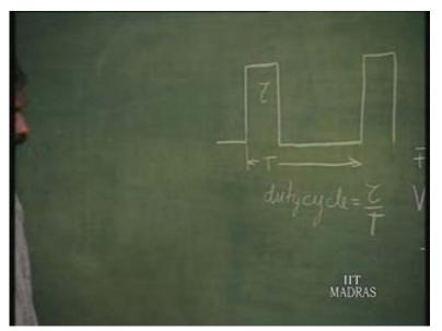
So, if such is the waveform which is appearing here because switch is closed for tau. Therefore, this is V i and when it is open, we want the...this voltage to be zero. That is done...instead of using another switch, we can as well use a diode which, because of the fact that the current in the inductor cannot change suddenly, as the switch is open, the current will continue to flow and that current will make the diode conduct and retain the potential equal to zero, ideally.
