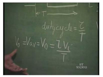
In a regulator, this converter can be used to get an output voltage which is always less than input voltage and maintain constant by adjusting tau over T. So, that is going to become a switched mode regulator. So, switched mode regulator is nothing but a converter with the duty cycle being controlled depending upon whether the output voltage is decreasing below reference value or increasing.
