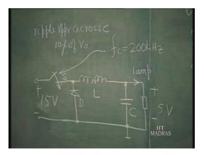
So, 10 percent of V naught is a reasonably acceptable value, let us say. That means peak to peak ripple is going to be 1 by 10 of 5 volts. Peak to peak ripple therefore is going to be one-tenth of 5 volts. So, this is going to be point 5 volts. That will be acceptable across the capacitor.
