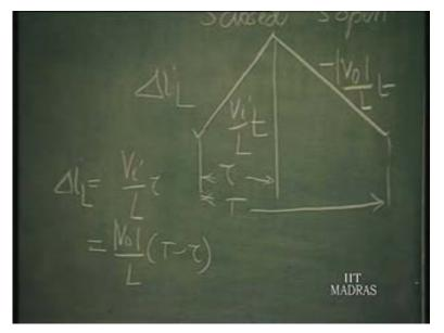
So, from this we get V naught by V i is equal to T minus...sorry. V i into tau. So, tau by T minus tau. So, tau and T minus tau can be greater than 1 or less than 1; and therefore, V naught can be greater than V i or less than V i or equal to V i because when tau is equal to T by 2, it is equal to V i.
