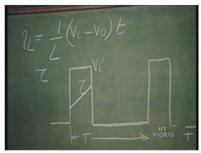
During this time, the switch is open; the current has already reached some value. So, this same current has to continue to flow and that current will force this diode to conduct. It will forward bias this diode and this voltage is going to maintain at zero, when the switch is open. So, this is zero and V naught is remaining same. That divided by L into T. That means current is going to decrease linearly with respect to time; that is determined by V naught by L, rate.
