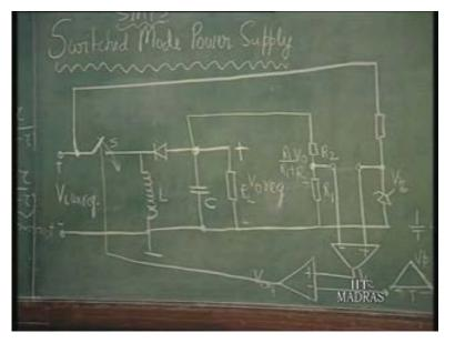
So, this is the complete schematic for a switched mode power supply. What additional things that is needed is a signal generator at the clock frequency; the typical clock frequency that is used for all these purposes is, nowadays, we can go up to megahertz. Earlier it was up to a 100 Kilohertz. Now, you can go even up to 1 megahertz.
