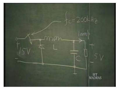
So, we have to design our converter, which means, we have to give the specification for L, C and the diode D and the switch S.
