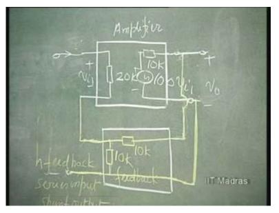
So, what you can obtain as this thing is 10 K and 20 K. Is it clear? So, this is 10 to the power of minus 4; this is again, point 5 into 10 to the power of minus 4 which is 1 point 5 into 10 to the power of minus 4. That many Siemens. This is...just a minute...Yes.
