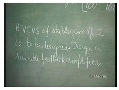
What should be the type of feedback? We are designing V C V S. The parameter that is ultimately of use is the g parameter. The type of feedback is obviously h feedback.
