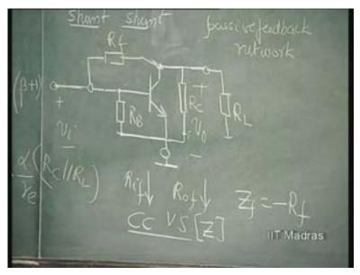
So, let us therefore see how it is going to become this. How do we therefore represent the feedback amplifier, composite amplifier, in terms of the composite Y parameter?
