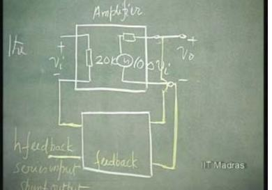
This should be passive and I want a gain of 2. That means, we have seen that, ideally speaking, if I want a gain of 2, I should have a feedback factor of half because we have seen in our earlier expression, if the loop gain is high, the g f is going to be 1 over the feedback factor. This we have seen. So, gain is required to be 2. That means we have to have a feedback of half.
