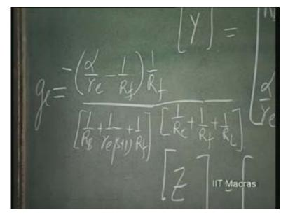
Now, there is no problem in this being negative as long as this whole quantity is remaining negative. That means Alpha over r e should be always greater than 1 over R f.
