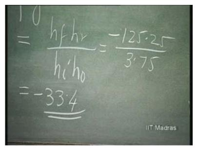
So, this is indicating that it is negative feedback. The value of this should be negative. So, it is negative feedback and it should be much greater than 1. Then only the feedback is effective. If it is much greater than 1 and negative, then the negative feedback is very effective. That means, it is definitely going towards its idealization.
