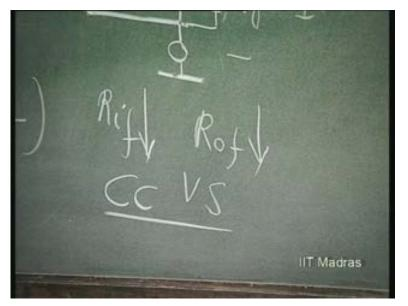
What is the parameter by which it can be represented? Since it is Y feedback, it can be represented by z parameter and what is the parameter that is going to become stabilized? Z f is going to be stabilized and Z f in this case is going to become equal to minus R f because Z f should become equal to some resistance which is coming as the feedback resistance. The only resistance that is coming back as feedback resistance is R f. So, Z f should ideally become R f.
