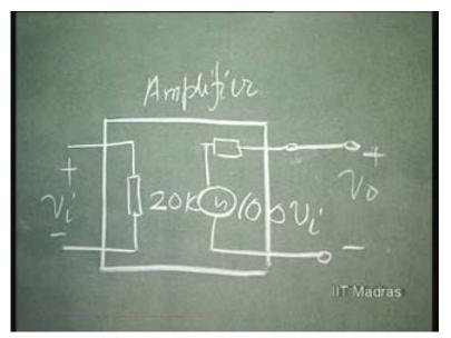
Now, we have to have the feedback for this. This is the feedback network which we are introducing. How are we introducing this? It should be in series at the input. So, I put it in series and it should be in shunt at the output. That is, output voltage is common to both; input current is common to both. And when it is in series, input current is common; when it is in shunt, output voltage is common. So, what is the feedback network?
