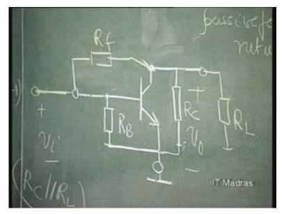
So, how is it at the input? How is it at the output? This is to be understood. I have not disturbed the earlier input voltage. I have not disturbed the earlier output voltage. So, I have connected the output to the input. That means, it can only be in shunt at the input and in shunt at the output.
