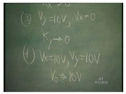
So, these are the four adjustments that have to be made in the case of a precision multiplier before it is ready, and we can say that V naught therefore is going to be equal to V x V y by 10. So, once you say that, thereafter, you do not have to keep telling that this multiplier is usable for a dynamic range of V x V y less than 10 volts, greater than minus 10 volts. All these things are understood.
