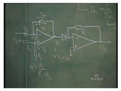
So, we have here an Alpha also coming into picture. That is to take care of V T variation with respect to temperature. So, V T by Alpha becomes independent of temperature over the range you desire.
