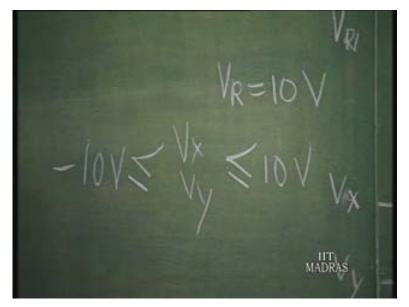
That means, if V x is 10 volts, V y is 10 volts, V naught is going to be 10 volts, if you select V r as 10 volts. So, that means this multiplier is compatible with another multiplier which is having the same dynamic range. So, we can couple these multipliers without any difficulty and have no problem about dynamic range of such things. That is why this has been standardized.
