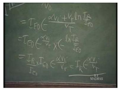
Once you code it in log form and then do the processing, and then you can do the decoding; so that whatever is occurring in the log form comes out of log form, gets expanded and comes in the normal form. So, this is what is normally done in the so-called antilog amplifier.
