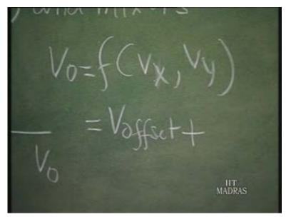
So V offset. Then, plus... In general, we can have what is called K x which is an output only due to V x. In the case of an amplifier, this is important; and it will be also similarly dependent upon V y. These are all linear terms which might exist, in general.
