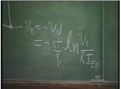
So, if I want to use this as a compandor, or use it as a log amplifier, I have to compensate for temperature variation here as well as here. Now, this temperature variation is a well-known thing. Why? This temperature coefficient of V T is K over q. It is constant. So, I can design a circuit using resistive network such as to exactly get the same temperature coefficient for that resistive network but in the opposite direction.
