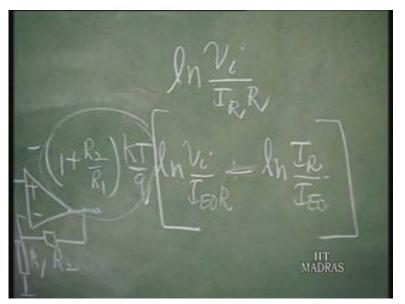
That means, this particular transistor again has to be connected as a diode here. So, it will be something like this. Let us say, it is connected as a diode and I had to pump in current into this so as to forward bias this by a current source which is going to be carrying a current of I R.
