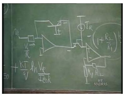
So, you can see that this is the way I will compensate for I E naught. That means the whole thing now is going to boil down to a nice logarithmic amplifier where it is going to be independent of temperature variation.
