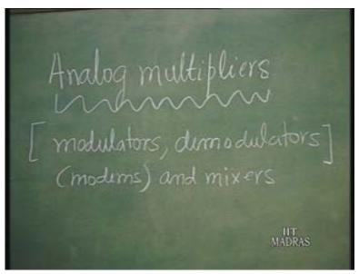
So, in this, the most important block is what is called as analog multiplier. Multiplier here means I am multiplying two currents or two voltages. It is not multiplication by a constant, which was the linear operation we discussed as amplifier or attenuator, earlier. Here, here it simply means multiplication by two voltages or currents.
