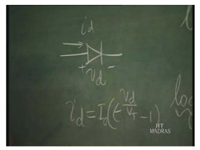
This is approximately equal to...if it is remaining in forward exponent V diode by V T, because its characteristic only in the forward bias region is going to be exploited for logarithmic operation. For therefore current switch, this I naught may be of the order of picoamperes or so. So, this under normal bias conditions is going to be something like this, approximation.
