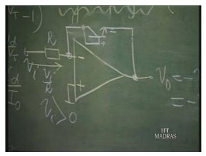
Instead, I can remove this and also connect it to ground. Now, what is the voltage here? It is still zero because this is ground potential and this is virtual ground potential, because of the op-amp. So, whether it is physically shorted or connected in this manner, the transistor is still acting at V c b equal to zero.
