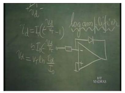
We know that this op-amp, if it is now connected in the feedback loop like this...and we take this output voltage V naught...this should always remain forward biased. That means, the current in this direction should keep flowing because that current alone can keep the diode in the forward bias mode. So, what is the current here? If this is V i, and if V i is greater than zero, then only the current direction is going to be this.
