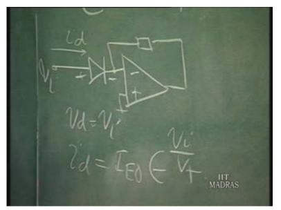
If V i is V T log something, this will become antilog. So, this is the antilog operation. Say, this current, when it is forced into a resistance R, will develop a voltage which is I d into R. So, V naught is equal to minus I d into R. This is plus, that is minus. So, we get this as minus R I E naught exponent V i by V T. This is the antilog operation or this is the data expandor.
